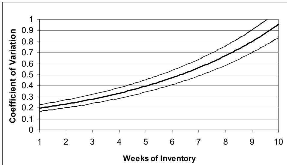
Figure 5. Relationship between coefficient of variation of demand and inventory required to achieve a 95 percent service level with 95 percent confidence limits.
