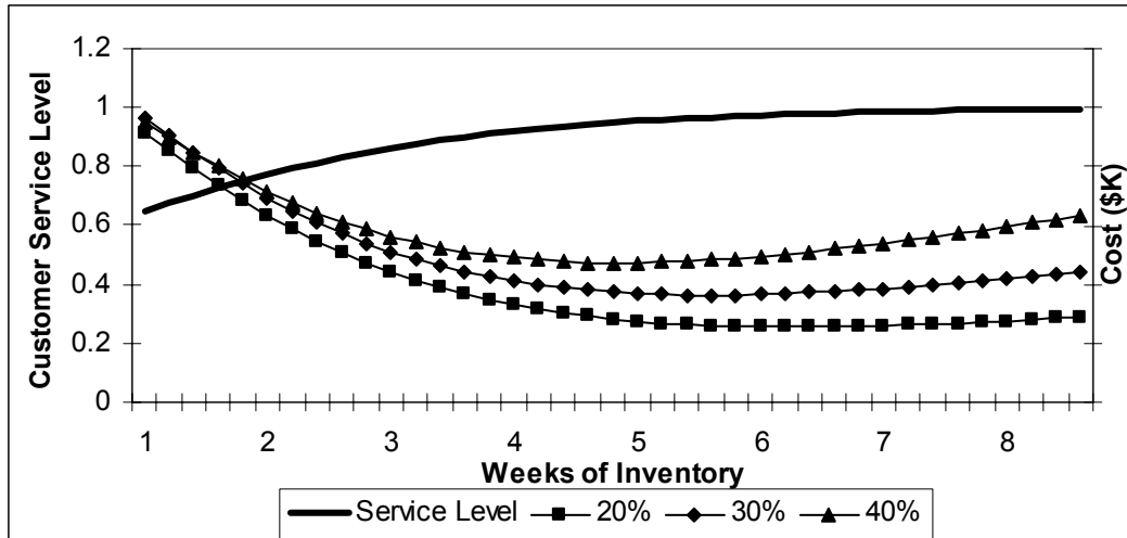
Figure 6. Sensitivity Analysis on the Effect of Product Margin on Ideal Service Level
