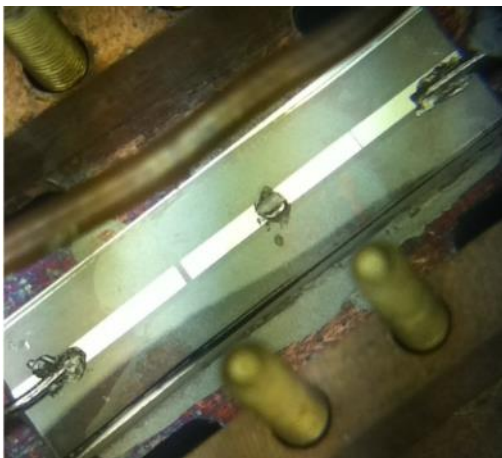
Figure 4.10 – (top) Autocad design of a 7 GHz Nb-on-Sapphire superconducting resonator. The meandering path allows for low frequency devices which fit within a smaller footprint. The long dimension of the entire pattern is 2 cm. (Bottom left) Photograph of a microstrip style Nb resonator with a sample. (Bottom right) The housing box used for mounting samples and measurements in our cryostat/dilution refrigerator. By an exclusively copper construction, the device/sample space within is free of any superconducting material that might lead to parasitic resonances.
