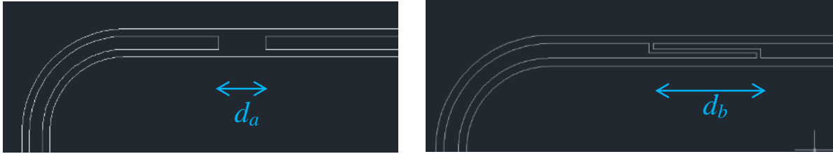
Figure 4.7 – Detail of the schematics showing the different styles of coupling gaps employed, with direct gaps shown in the left and interdigitated gaps on the right.
