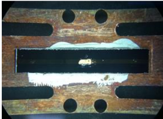
Figure 4.2 – (top left) Photograph of the pulse circuitry used to perform pulsed microwave measurements. (top right) Circuit diagram of the pulse delivery and homodyne detection instrumentation. Table 1 contains a description of the items indexed by their alphabetical labels. (bottom left) Photograph of a sample mounted on a 10 GHz Au resonator, which is in turn mounted on the bottom plate of our Cu housing box. The housing box can be mounted into our cryostat/dilution refrigerator with contacts between coaxial microwave lines and the feed lines of the device. (bottom right) Spin echo signal from a “Bruker Coal” sample at 4.3 K. The solid lines are the signal after subtraction of a background, with different colors representing a different time delay between \pi -half = 120 ns and \pi = 240 ns pulses. The dotted red line is an exponential fit to the echo peaks, extracting a spin-spin relaxation time of 1.3 \mu s.
