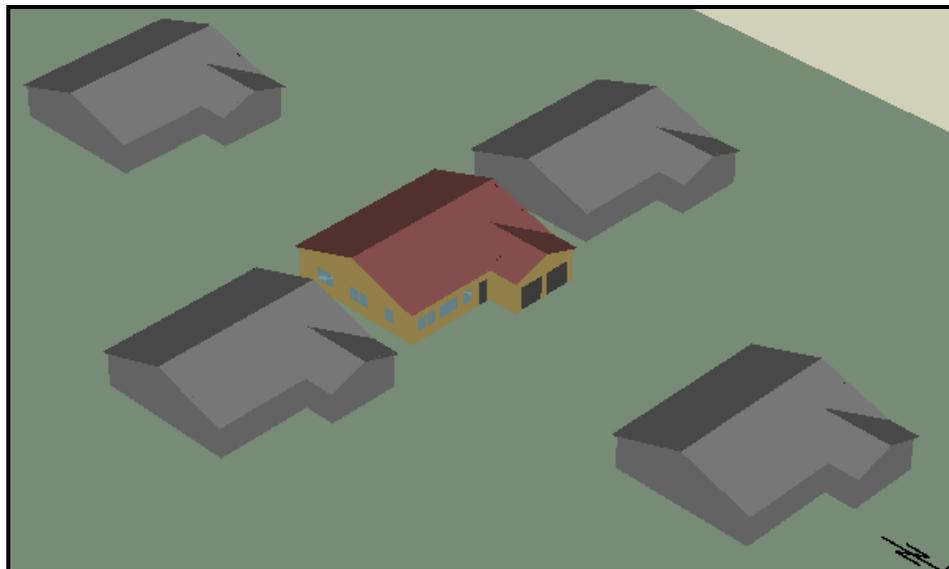
Figure 4. Prototypical 1,790 ft<sup>2</sup> residence rendered in BEopt/EnergyPlus with adjacent buildings
