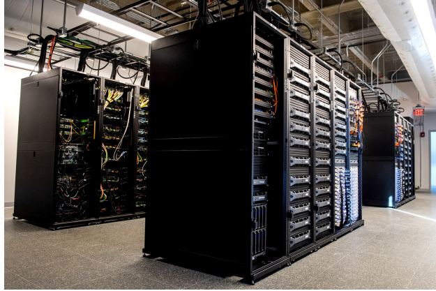
Figure 3.1: Colosseum [3]: High-performance USRP devices arranged in stacks known as ‘quads’.
