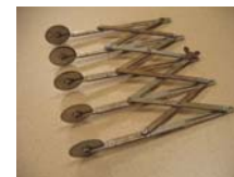
Dough divider— used for cutting dough into even strips
