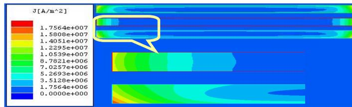
Figure 3.5 Proximity effect (three layers in parallel).
