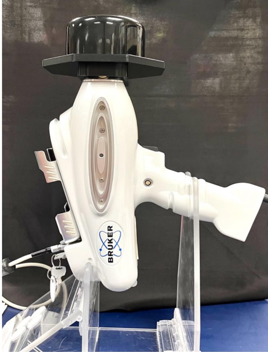
Figure 3: Bruker HHXRF positioned in acrylic stand (Image by Griffon Binkowski)
