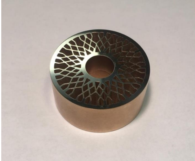
Figure 45 Demonstrative Component Manufactured by LPBF of Cu10Sn10 (Power=350W, Scan Speed=750mm/s, Hatch Space=0.12mm) Double Layered Pipe (~5 cm in Diameter) with Internal Cooling Channels and Grit-blasted Surface Finish
