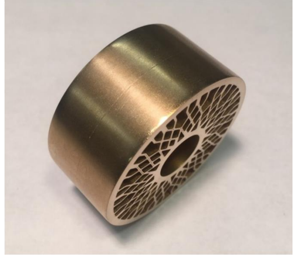
Figure 45 Demonstrative Component Manufactured by LPBF of Cu10Sn10 (Power=350W, Scan Speed=750mm/s, Hatch Space=0.12mm) Double Layered Pipe (~5 cm in Diameter) with Internal Cooling Channels and Grit-blasted Surface Finish
