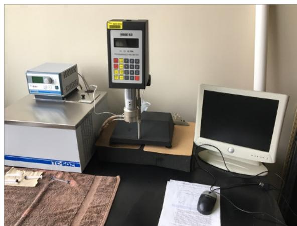
Figure 2. Cone/Plate Rheometer Used
