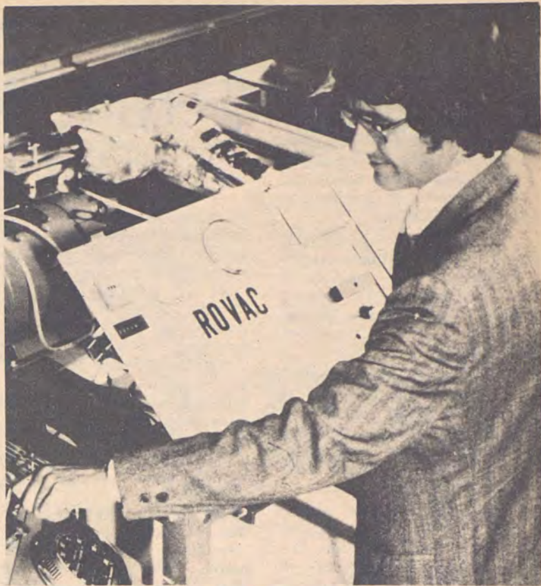
DR. THOMAS Edwards of the engineering department demonstrates the ROVAC system of air-conditioning that converts air into a refrigerant and eliminates the use of freon gas. This unit, Edwards' invention, is to be installed in a Chrysler Corp. test car.
