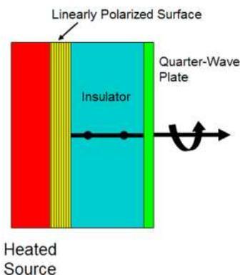
Fig. 4. Compact, multi-layer circular polarizer for emitted radiation.
