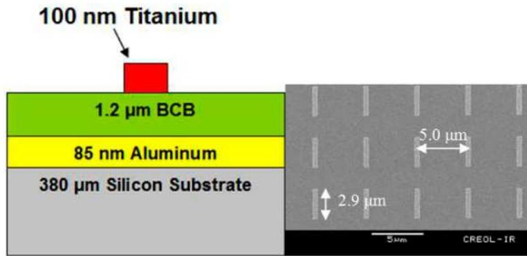
Fig. 1. Schematic of a unit cell of the dipole array and a scanning electron micrograph of the fabricated array with array dimensions labeled. The width of the dipoles is  $0.5 \mu\text{m}$ .
