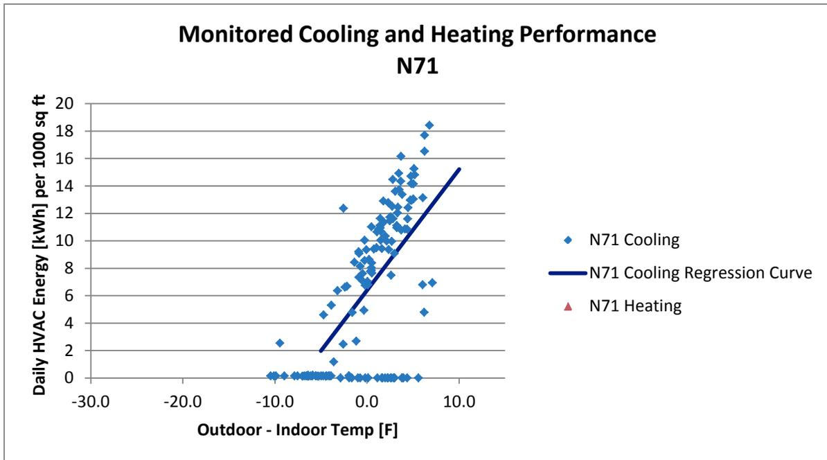
Figure A-75 Monitored Cooling and Heating Performance, N71
