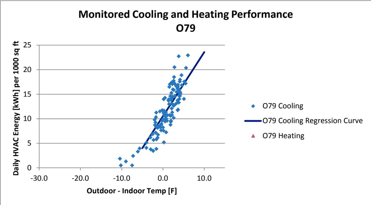
Figure A-214 Monitored Cooling and Heating Performance, O79
