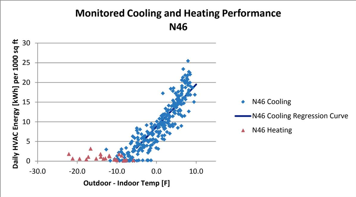
Figure A-47 Monitored Cooling and Heating Performance, N46
