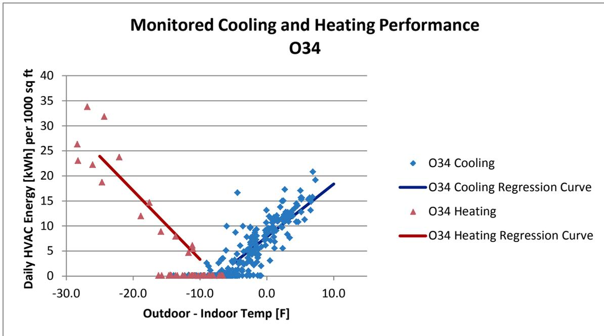
Figure A-145 Monitored Cooling and Heating Performance, O34
