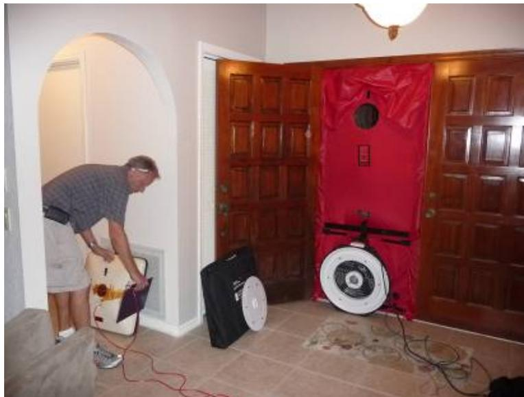
Figure 4-28. Blower Door set up in exterior doorway in preparation for house tightness and duct pressure pan tightness testing.
