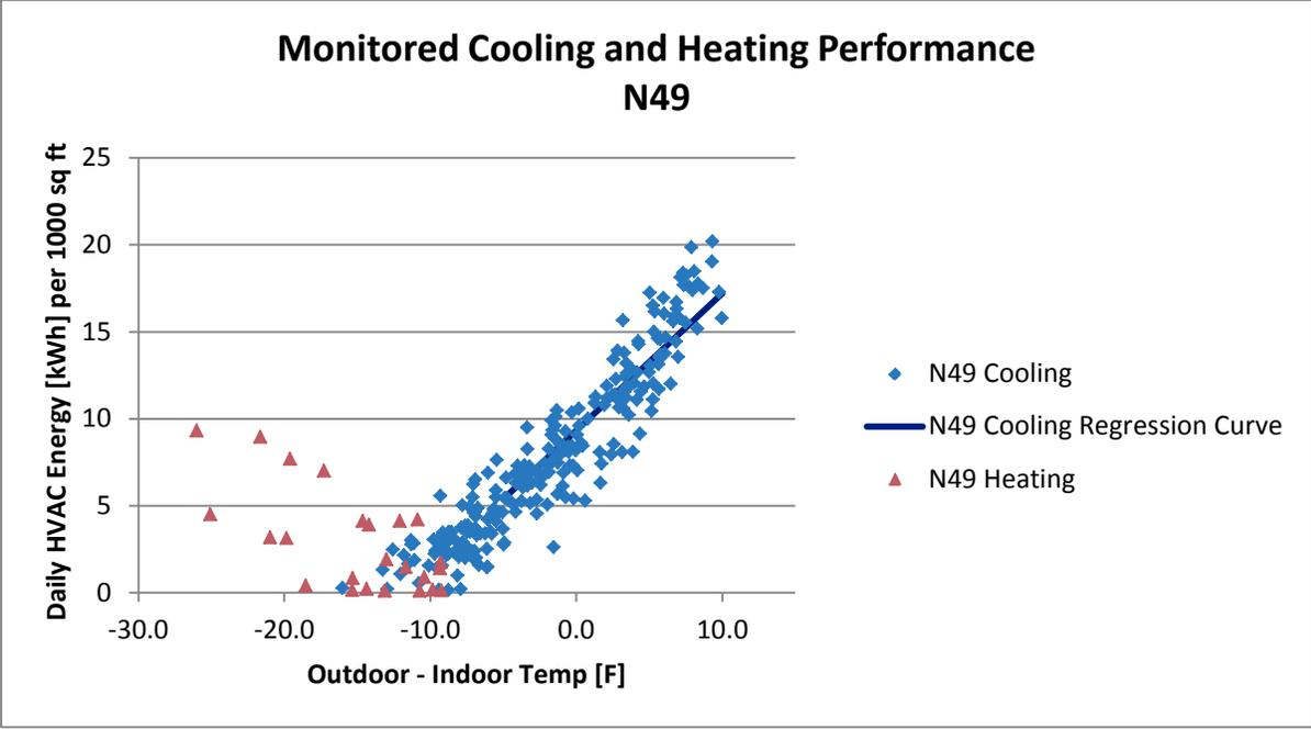
Figure A-56 Monitored Cooling and Heating Performance, N49
