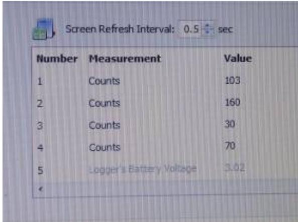
Figure 4-6. Photo of logger screen while connected to the laptop that shows initial pulse count at beginning of evaluation period.
