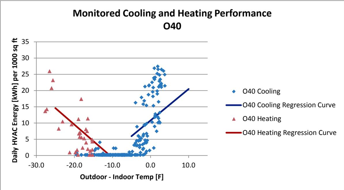
Figure A-162 Monitored Cooling and Heating Performance, O40
