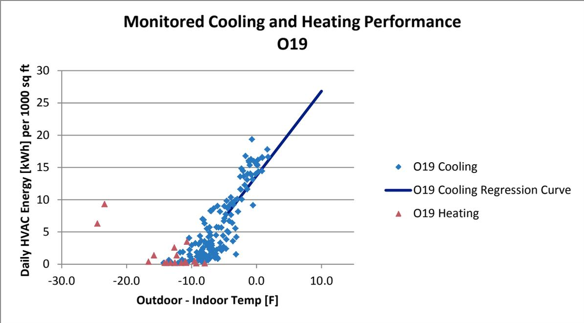
Figure A-123 Monitored Cooling and Heating Performance, O19
