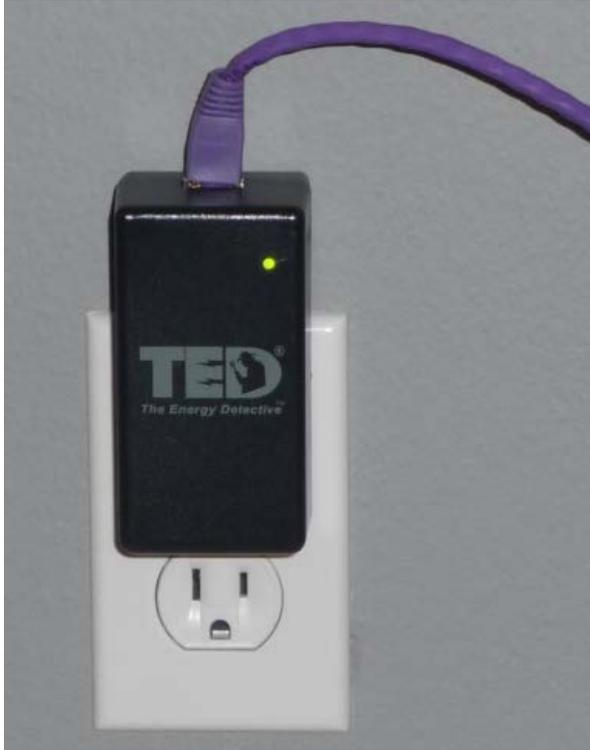
Figure 4-1. A TED energy data logger (gateway). The unit collects and stores data which can be accessed by internet using an ethernet connection. Current and voltage sensors called MTUs are located inside the electric service panel.
