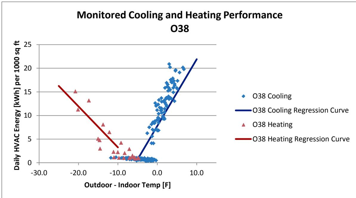
Figure A-156 Monitored Cooling and Heating Performance, O38
