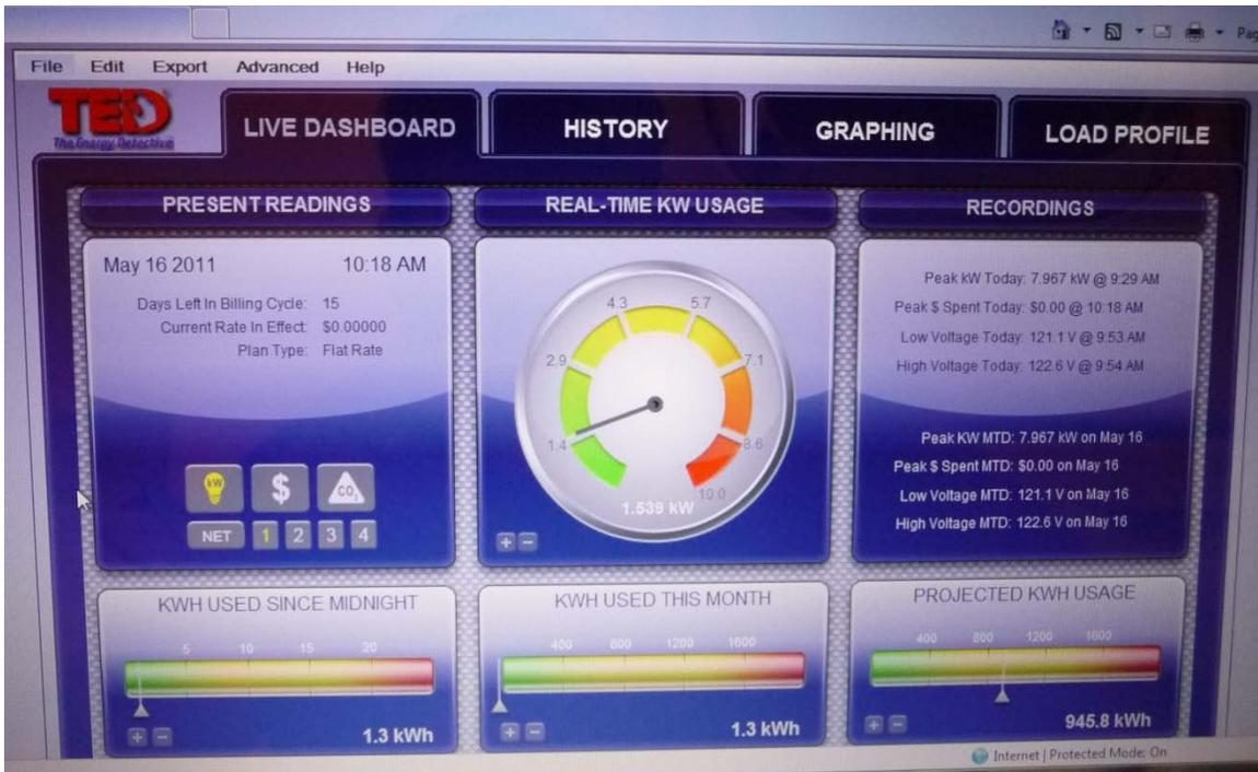
Figure 4-3. View of TED energy monitoring showing whole house power during an installation. This portal is used to look at live data and download stored data.
