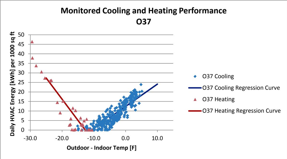
Figure A-153 Monitored Cooling and Heating Performance, O37
