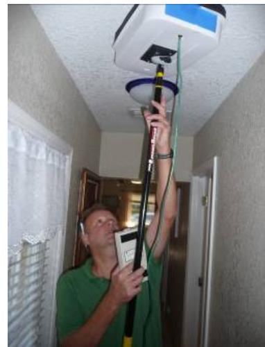
Figure 4-30. PPan measurement at a supply grill located in hall ceiling below attic space.
