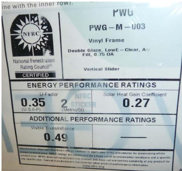
Figure 4-10. Example of an NFRC window rating tag showing U and SHGC values.
