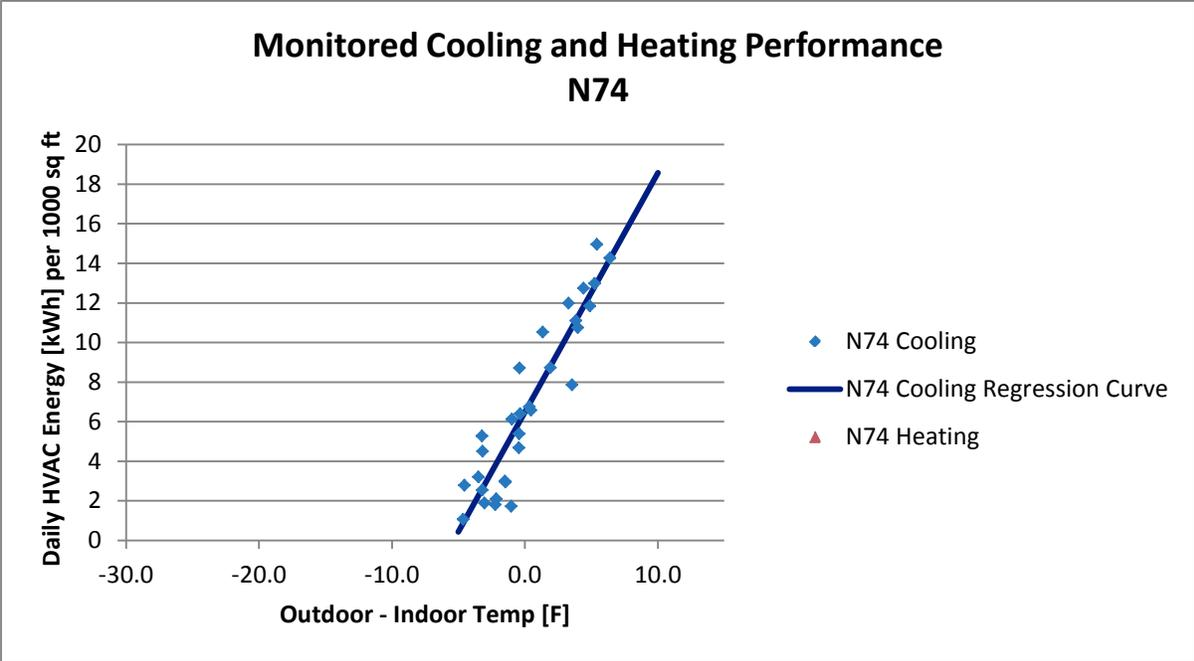
Figure A-81 Monitored Cooling and Heating Performance, N74
