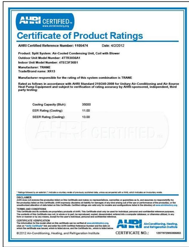
Figure 4-25. Model numbers from the outdoor and indoor unit are looked up on the AHRI directory of efficiency ratings to determine the heating and cooling efficiency. This unit is a straight cool system with strip heat so only the cooling is rated. This air conditioner has a 13.0 SEER rated efficiency.
