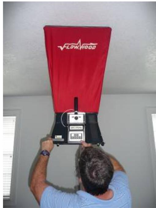
Figure 4-32. Airflows were also measured using a Flow Hood at return grills.
