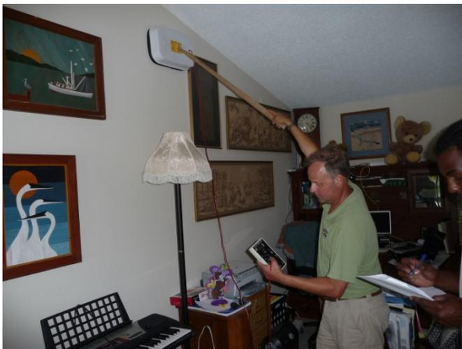
Figure 4-29. The pressure pan duct leakage test is used to indicate presence of significant air leakage near the supply and return grill measurements.
