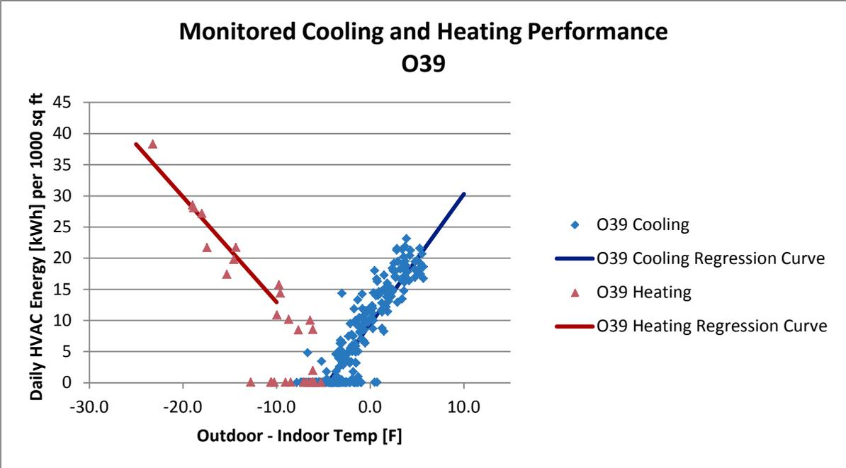
Figure A-159 Monitored Cooling and Heating Performance, O39
