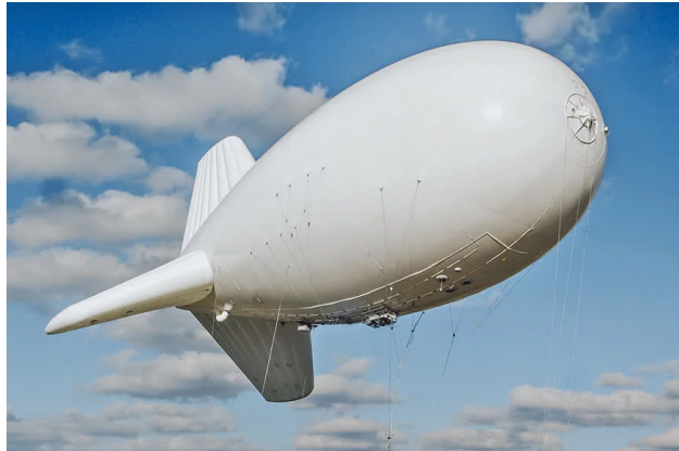
Figure 2.3: Tethered aerostat radar system [3]
