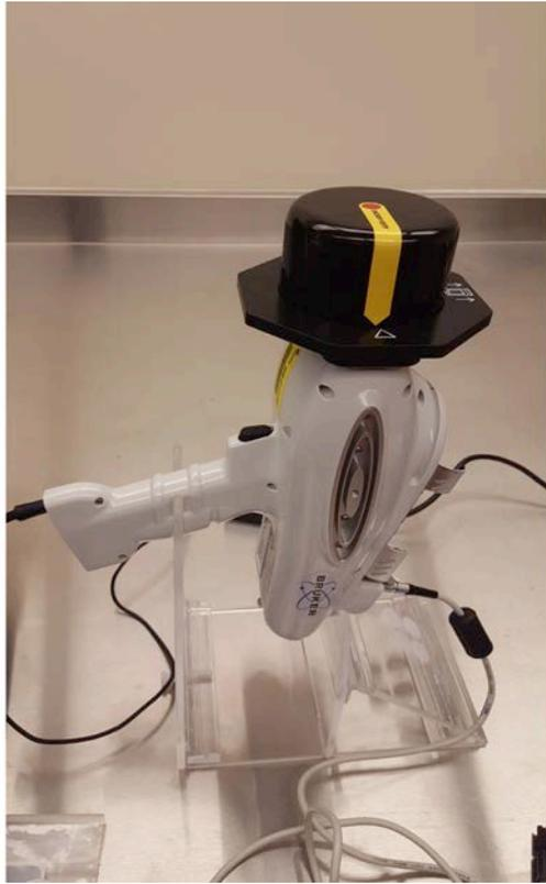
Figure 3: Handheld XRF Bruker Tracer III SD of University of Central Florida (Fertig, 2018)
