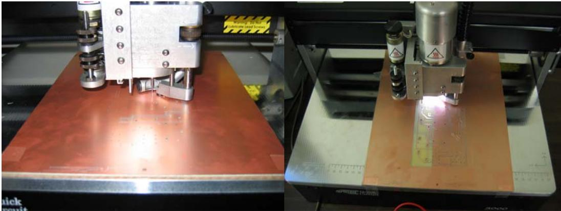
Figure 37: Milling Machine In Use
