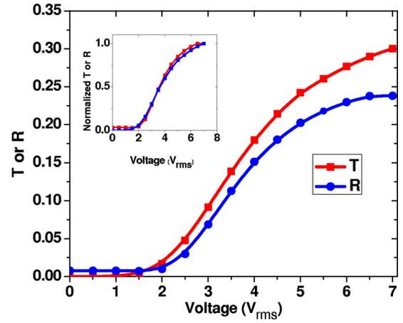
FIG. 3. (Color online)  $V_T$  and  $V_R$  curves for the proposed TR-LCD. The inset shows the normalized results.
