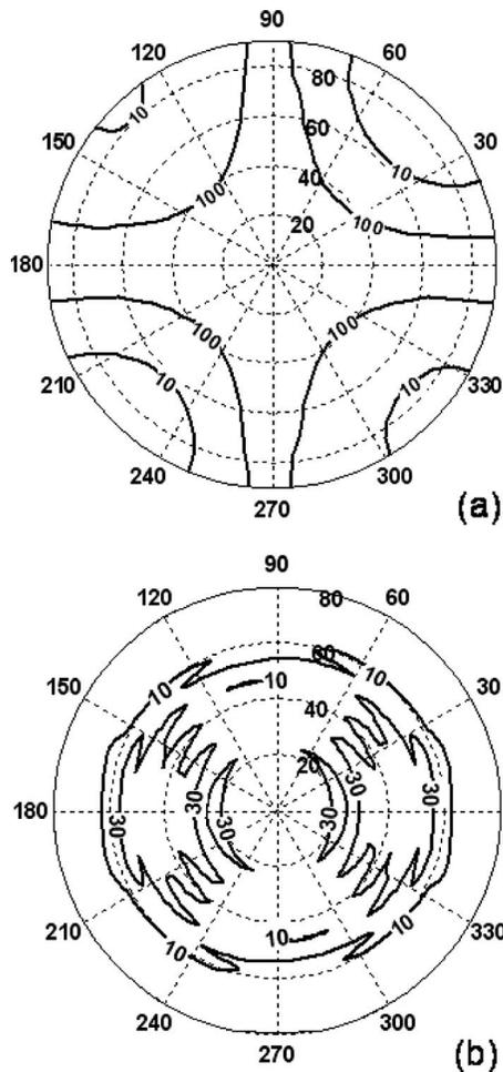
FIG. 4. Isocontrast plots for (a)  $T$  mode and (b)  $R$  mode of the proposed TR-LCD.
