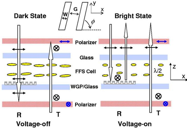
FIG. 2. (Color online) Working principles of the  $T$  and  $R$  modes at both dark (voltage off) and bright (voltage on) states.
