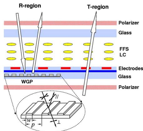
FIG. 1. (Color online) Schematic structure of the single cell gap FFS transmissive LCD device using embedded wire grid polarizer as reflector.
