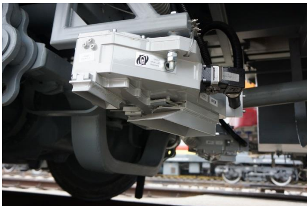
Figure 12: Rail profile inspection system installed on the car bogie
