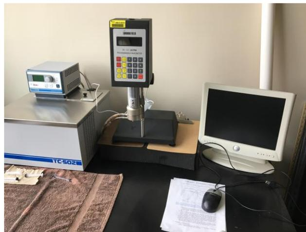
*Figure 2- Cone/Plate Rheometer Used*
