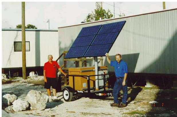
Figure 1: FEMA 500 Wp trailer
