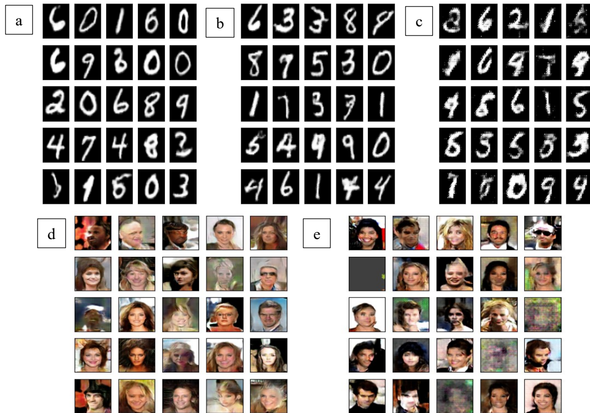
Figure 27. MNIST and celebA were trained from scratch on W32A32 for 100 epochs and resulted in (a) and (d) with an FID score of 49 and 104 respectively. Then, MNIST fine-tuned to a lower bit-width with more training epochs resulted in (b) W4A4 and (c) W1A2 with an FID score of 53 and 126 respectively. Finally, celebA is also fine-tuned to the lowest possible bit-width with more training epochs resulted in (e) W4A4 with an FID score of 129.
