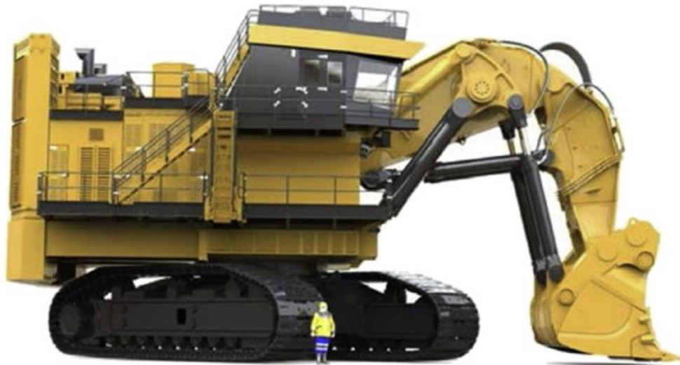
Figure 1.8: ~ 50 MJ electrochemical capacitor based energy storage system in the Caterpillar 6120 H FS 1400-ton hybrid mining shovel. Reproduced from Ref. 9
