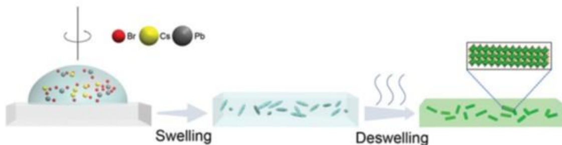
Figure 4.1: in situ synthesis of encapsulated CsPbBr 3 nanorods. Reproduced from Ref. 67 with permission from The Royal Society of Chemistry.
