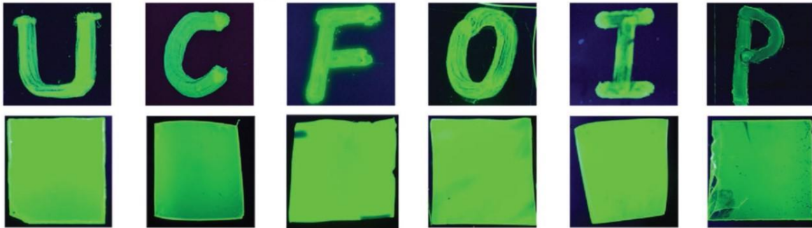
Figure 3.2: Cotton swab painting and spin coated samples with UV excitation (365 nm). Samples displayed from left to right are: MAPbBr 3 -PS, MAPbBr 3 -PC, MAPbBr 3 -ABS, MAPbBr 3 -CA, MAPbBr 3 -PVC, and MAPbBr 3 -PMMA. Figure adapted from reference [43].
