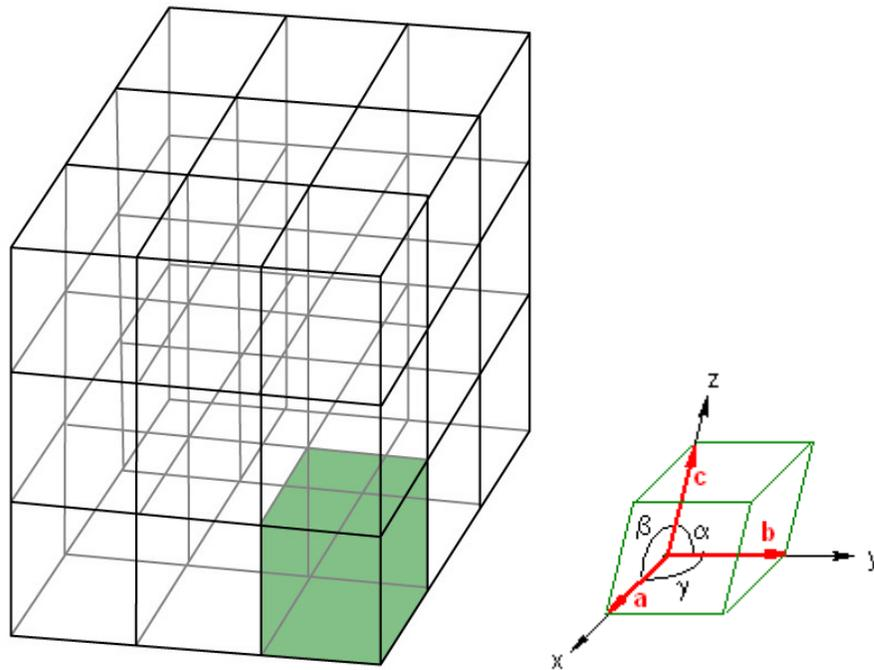
Figure 3. Cubic space lattice of an ideal crystalline (left) solid and the unit cell (right) [50].
