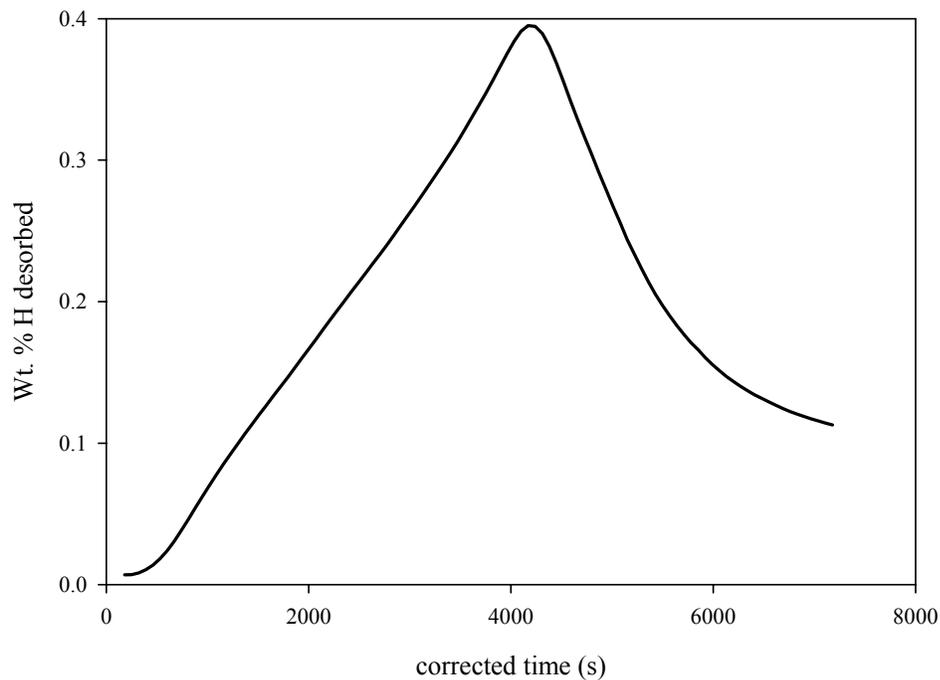
Figure 16: Percent hydrogen desorbed for dehydriding of VTiNi.
