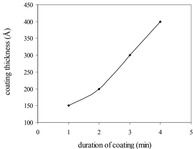
Figure 8. Coating thickness dependence on coating duration.
