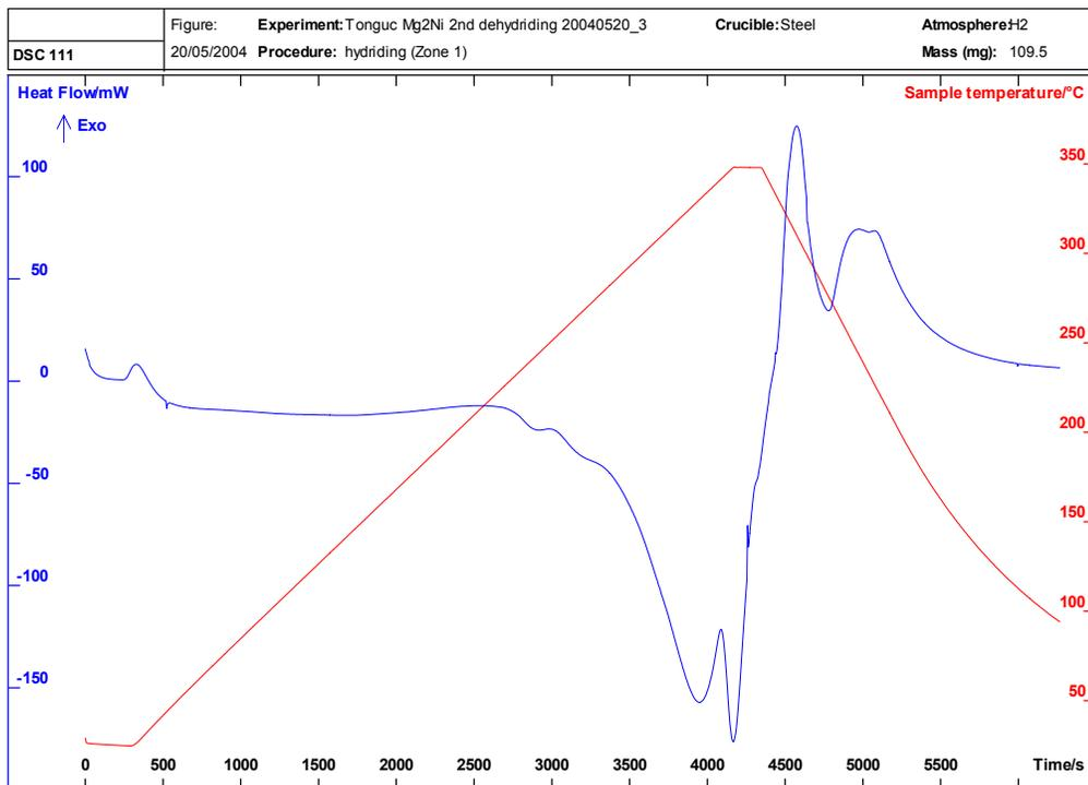
Figure 11: Thermogram for dehydriding of Mg<sub>2</sub>Ni.
