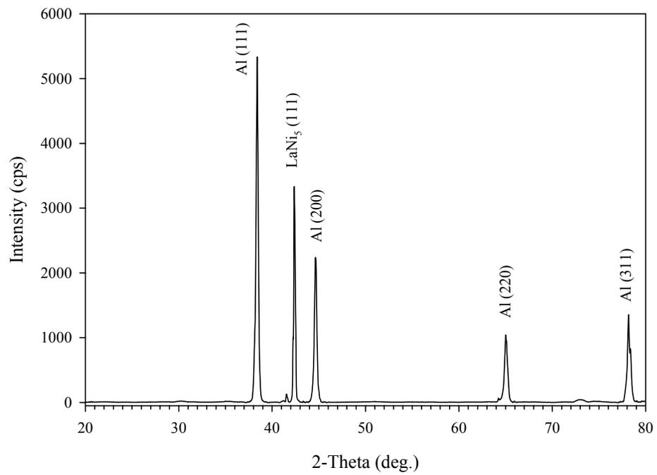
Figure 41. XRD spectrum of non-milled LaNi<sub>5</sub> with 33 mole % Al.
