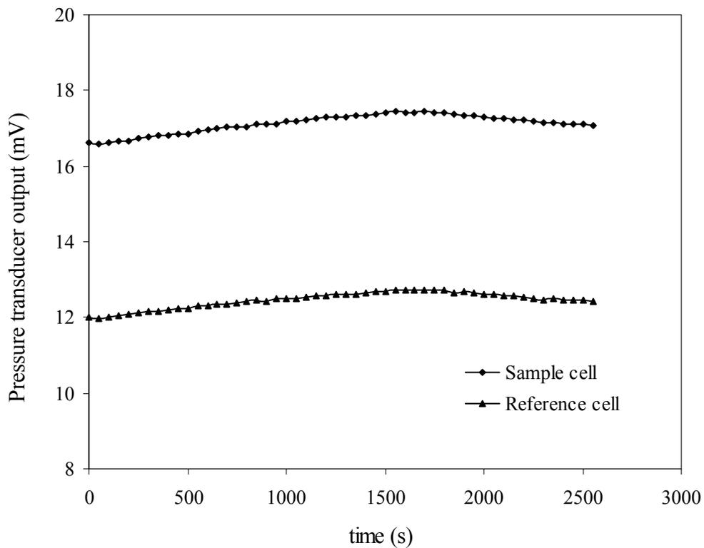
Figure 25: Pressure transducer output curve for VTiNi heated under He atmosphere.
