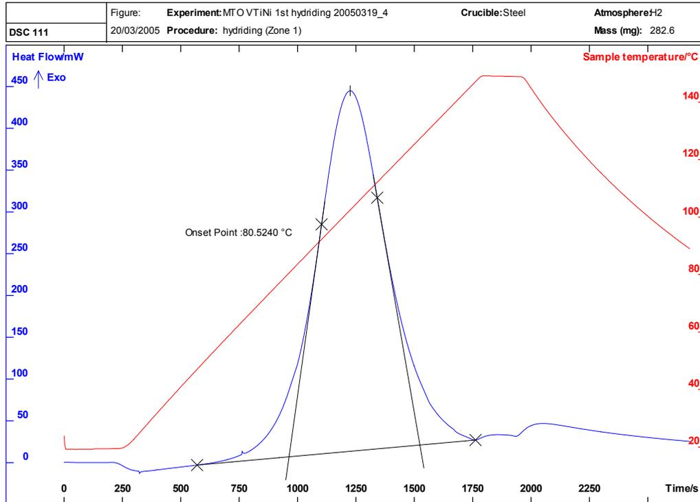
Figure 13: Thermogram for initial hydriding of VTiNi.
