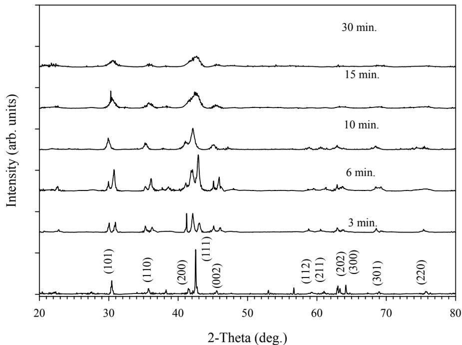
Figure 39. XRD spectra of LaNi<sub>5</sub> milled for varying durations.
