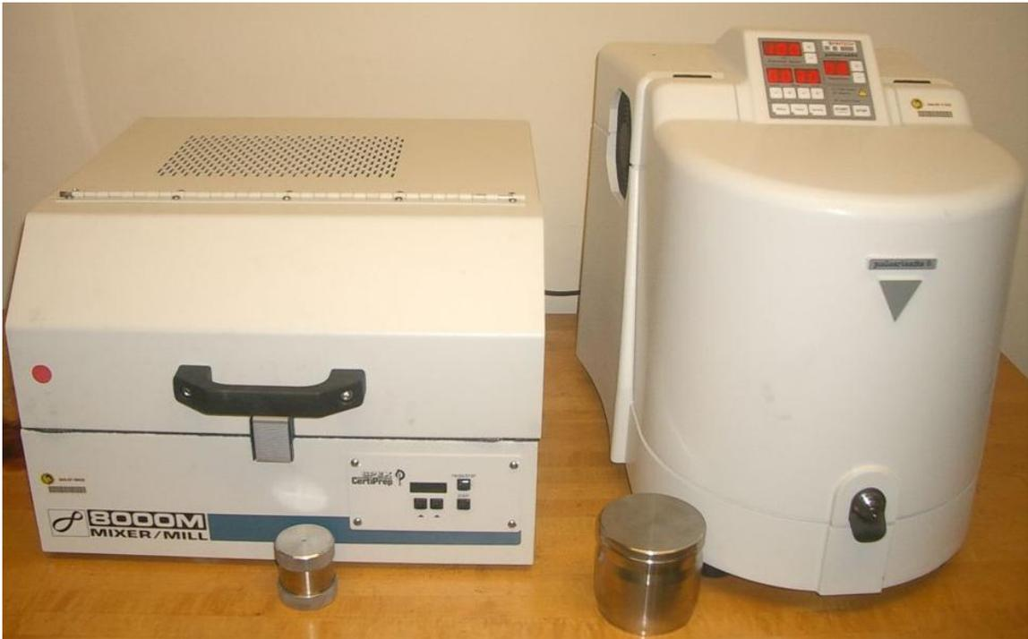
Figure 5. The high energy Spex 8000M Mixer/Mill (left) and the Fritsch Planetary Mill (right).
