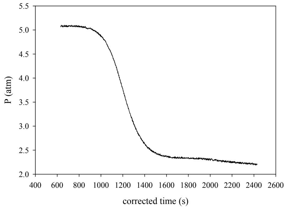
Figure 14: Composition and pressure curves for the initial hydriding of VTiNi.
