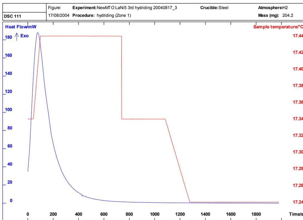
Figure 17: Thermogram of ball milled and thermally activated LaNi<sub>5</sub>.
