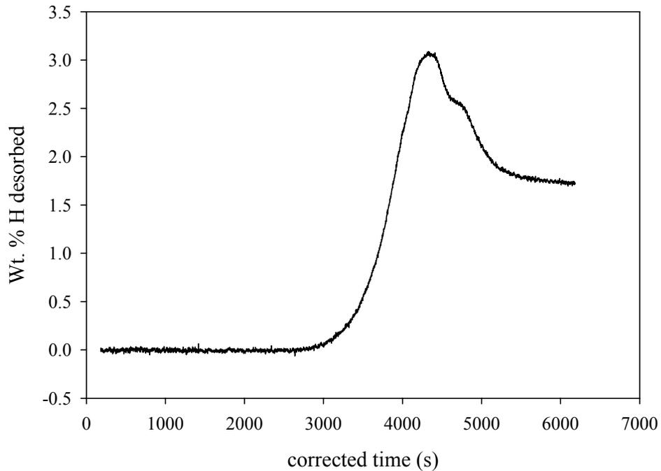
Figure 12: Percent hydrogen desorbed for dehydrating of  $Mg_2Ni$ .
