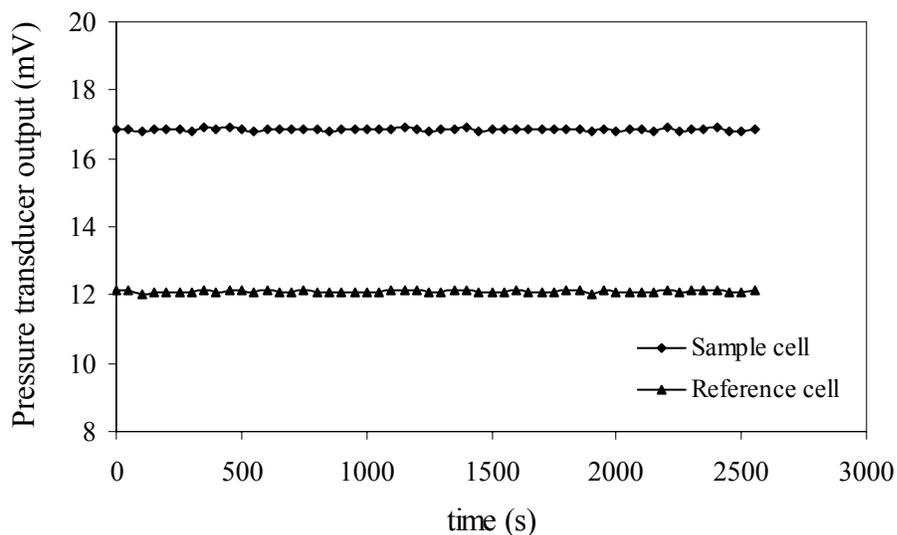
Figure 29: Pressure transducer output of DSC for 50 mole % Al in LaNi<sub>5</sub> under pure He atmosphere.
