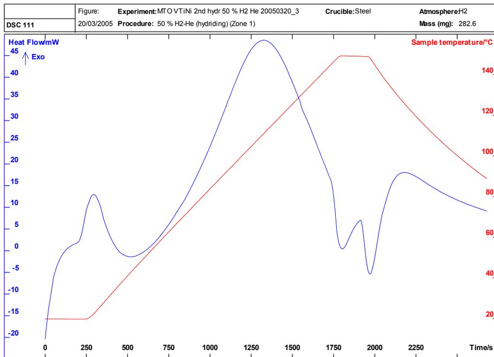
Figure 26: Thermogram of VTiNi hydrided with 50% (v/v) H<sub>2</sub>-He mixture.
