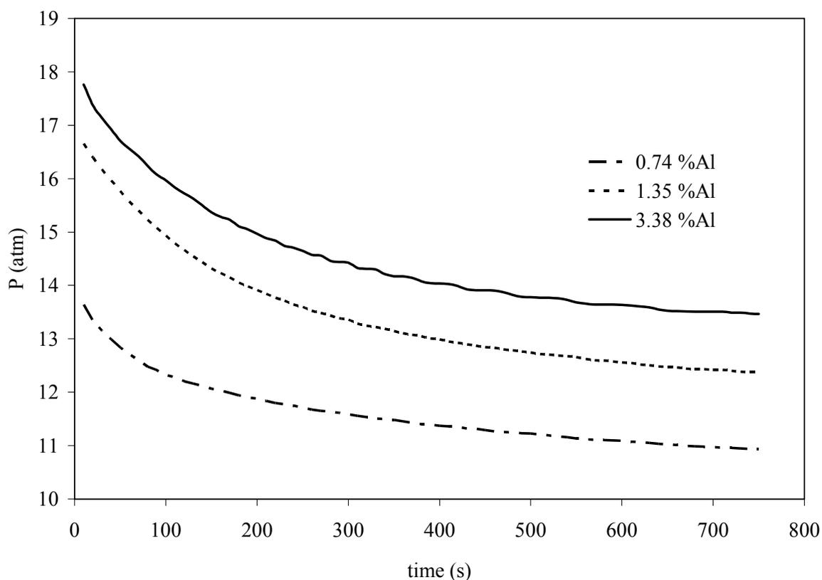
Figure 34. Pressure profiles under 50% (v/v) H<sub>2</sub>:He atmosphere.
