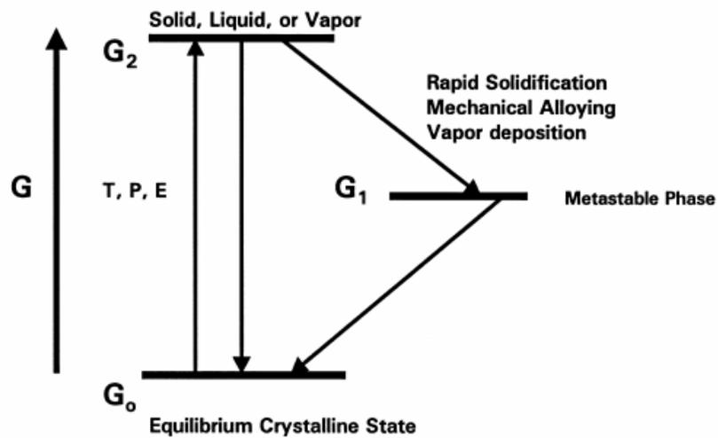
Figure 2. Energy diagram for metastable phase formation by mechanical alloying.
