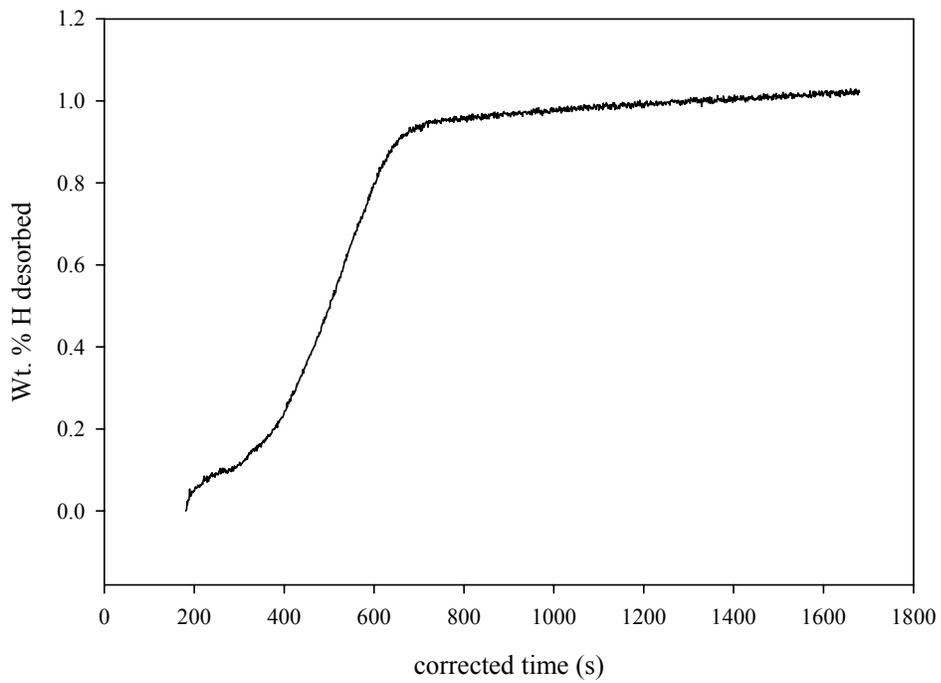
Figure 22: Percent hydrogen desorbed plot for dehydrating of LaNi<sub>5</sub>.
