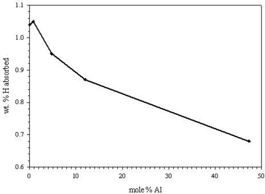
Figure 24: Percent hydrogen capacity as a function of mole % Al in LaNi<sub>5</sub>.
