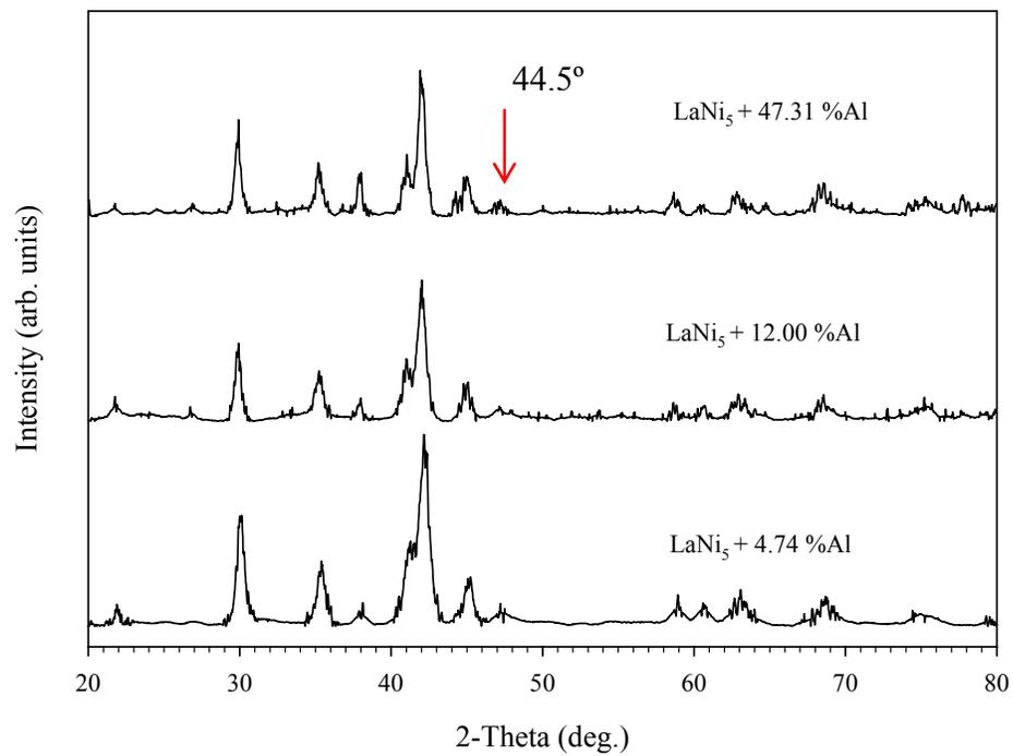
Figure 42. XRD spectra of milled  $\text{LaNi}_5$  containing Al.
