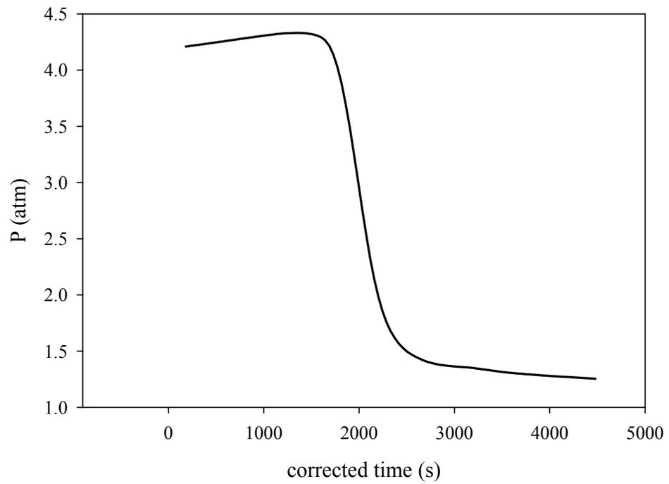
Figure 10: Composition and pressure plots for initial hydriding of  $Mg_2Ni$ .
