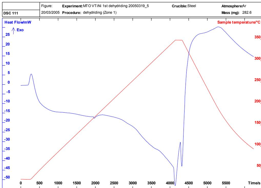
Figure 15: Thermogram for dehydrating of VTiNi.
