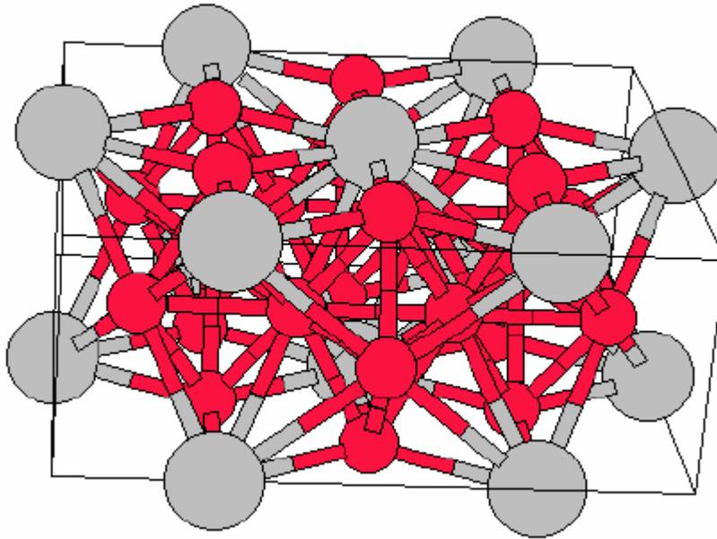
Figure 4. CaCu<sub>5</sub>-type P6/mmm structure of LaNi<sub>5</sub> [51]. Gray spheres indicate La atoms.
