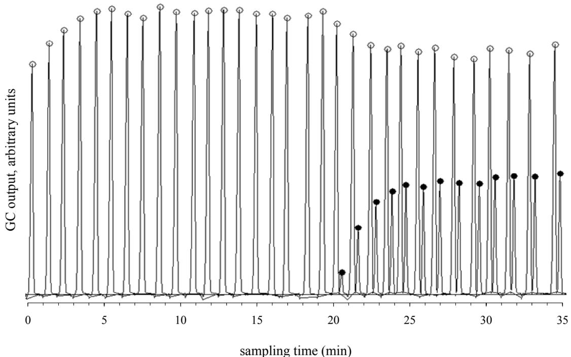
Figure 35. Chromatogram for hydrogen absorption in the U-tube reactor.
