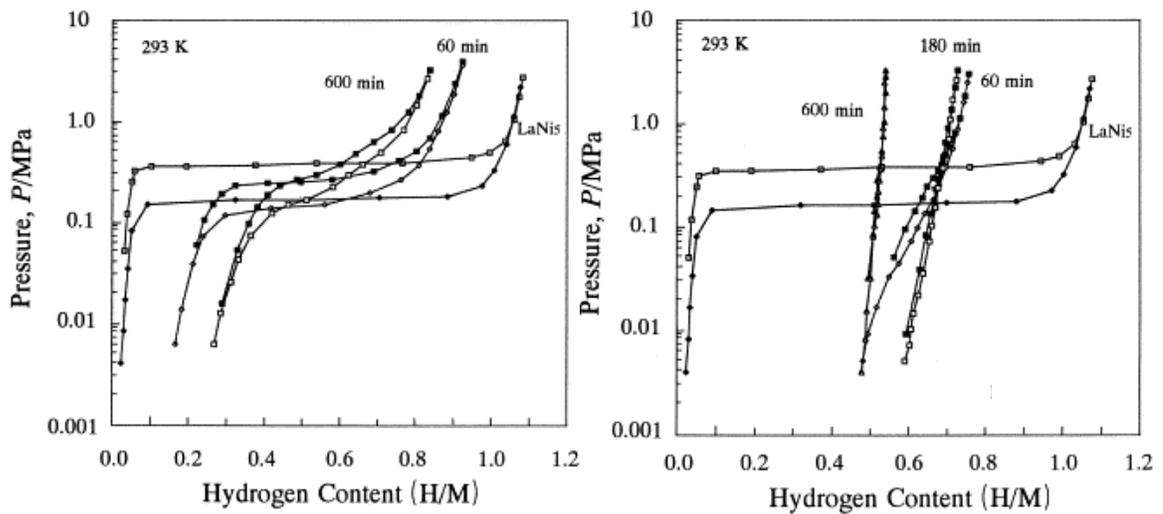
Figure 20. Effect of milling time on pressure-composition isotherms of LaNi<sub>5</sub> under argon (left) and hydrogen (right) atmospheres.
