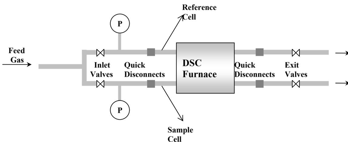
Figure 6. Schematic representation of the DSC setup. P denotes pressure transducer.
