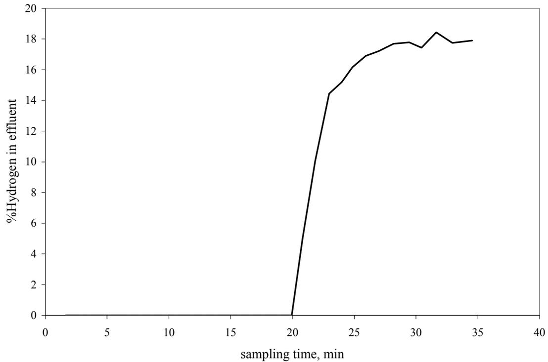
Figure 36. Effluent gas composition as percent hydrogen (v/v).
