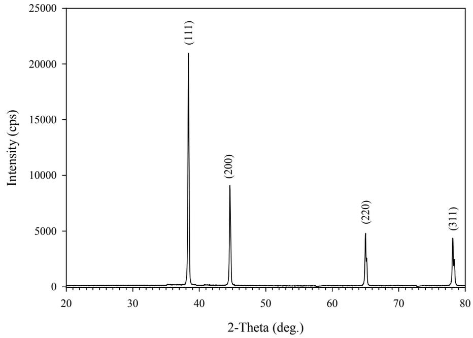
Figure 40. XRD spectrum of aluminum.
