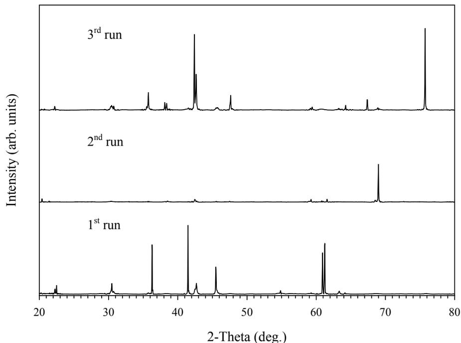
Figure 38. XRD spectra of  $\text{LaNi}_5$  ground with mortar and pestle.
