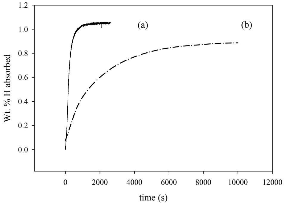
Figure 30: Percent hydrogen curves for LaNi<sub>5</sub> with 0.77% Al, hydriding under pure H<sub>2</sub> (a) and 50% (v/v) H<sub>2</sub>-He (b).
