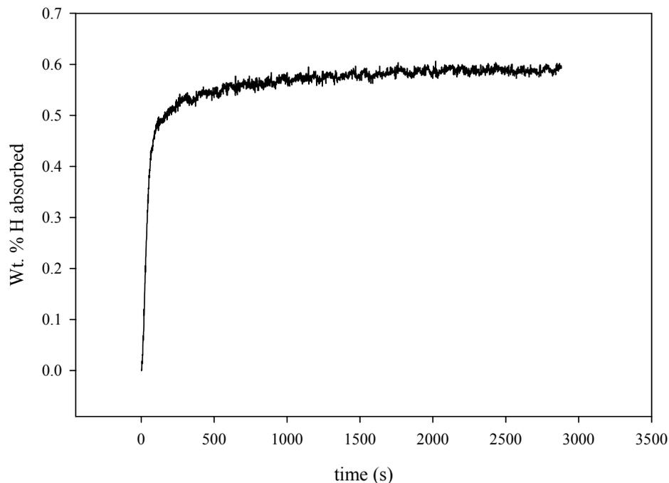
Figure 19: Composition curve for hydriding of  $\text{LaNi}_5$  prepared in Fritsch Pulverisette Mill at 300 rpm.
