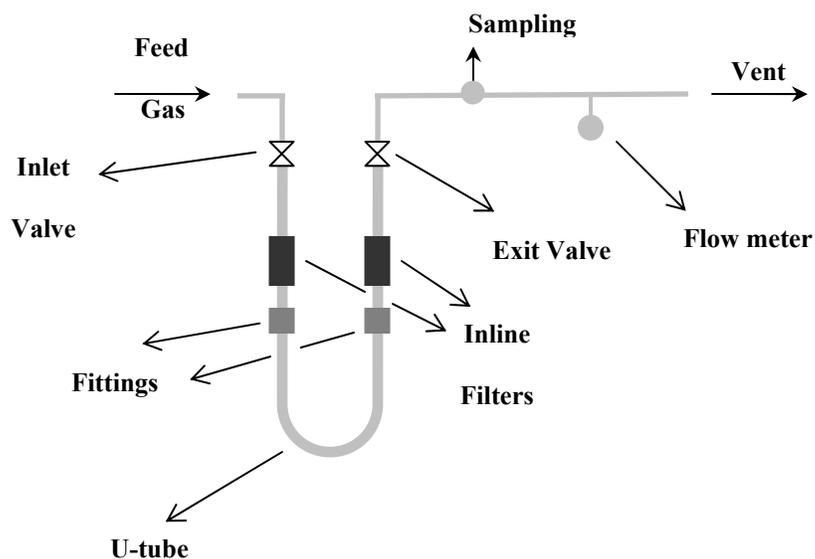
Figure 7. The U-tube reactor.
