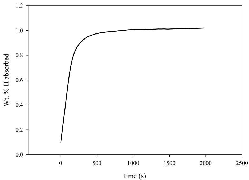
Figure 18: Composition curve of ball milled and thermally activated LaNi<sub>5</sub>.
