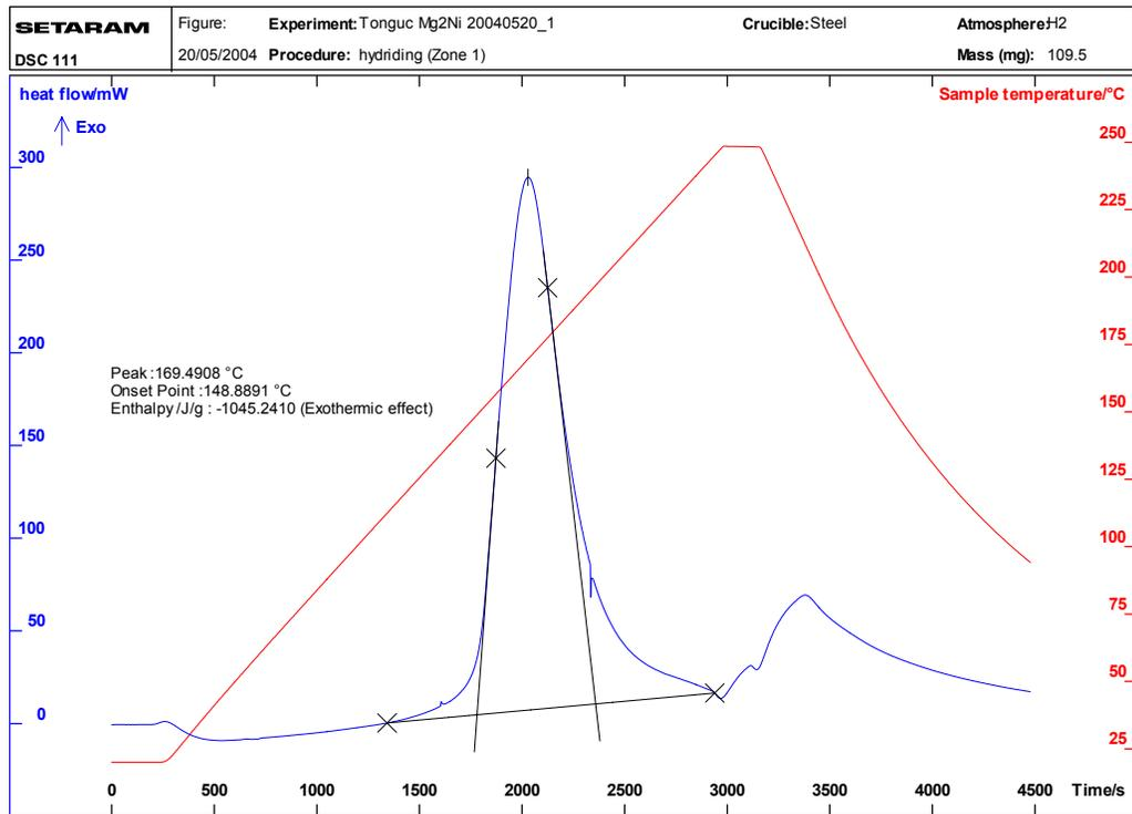
Figure 9: Thermogram for initial hydriding of Mg<sub>2</sub>Ni.
