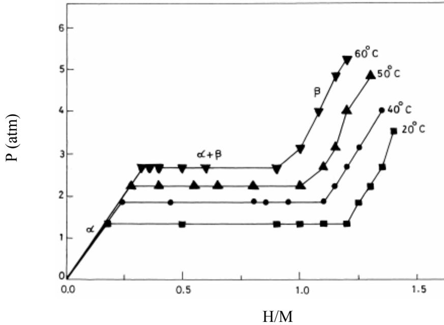
Figure 1. Pressure-composition diagram for  $LaNi_5$  [17].
