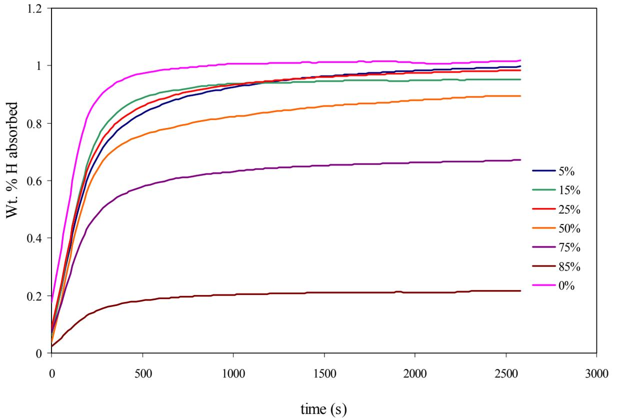
Figure 23: Percent hydrogen uptake curves for different amounts of Al in  $\text{LaNi}_5$
