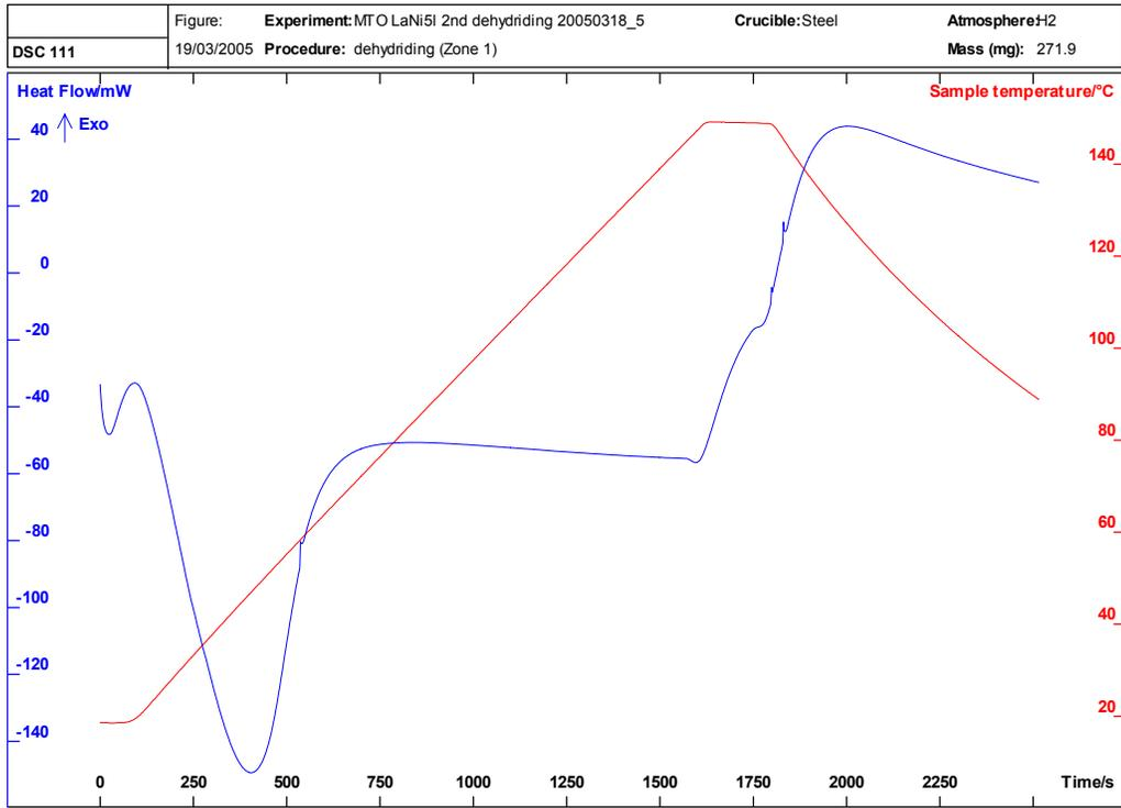
Figure 21: Thermogram for dehydrating of LaNi<sub>5</sub> starting with 1 atm. H<sub>2</sub>.
