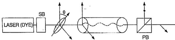
FIG. 2. Schematic showing how the seeded input into the fiber is obtained.
