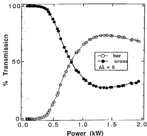
FIG. 3. All-optical switching between polarization states in a fiber filter tuned to the resonant wavelength. Power is input into the bar state only. SB and PB are the Soleil-Babinet compensator and the polarizing beam splitter, respectively.
