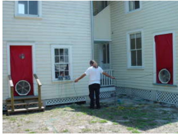
Figure 10 - Testing at the Rossetter home site required the simultaneous use of 2 Blower Doors
