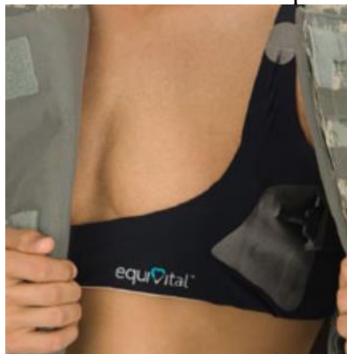
Figure 1. Equivital EQ02 Life Monitor - Sensors connect on the inside behind the grey patch, just on the side of the chest.
