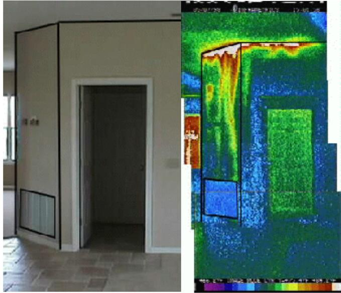
**Figure 2.** Thermograph of air being drawn from the attic to the air handler in a Florida house.
