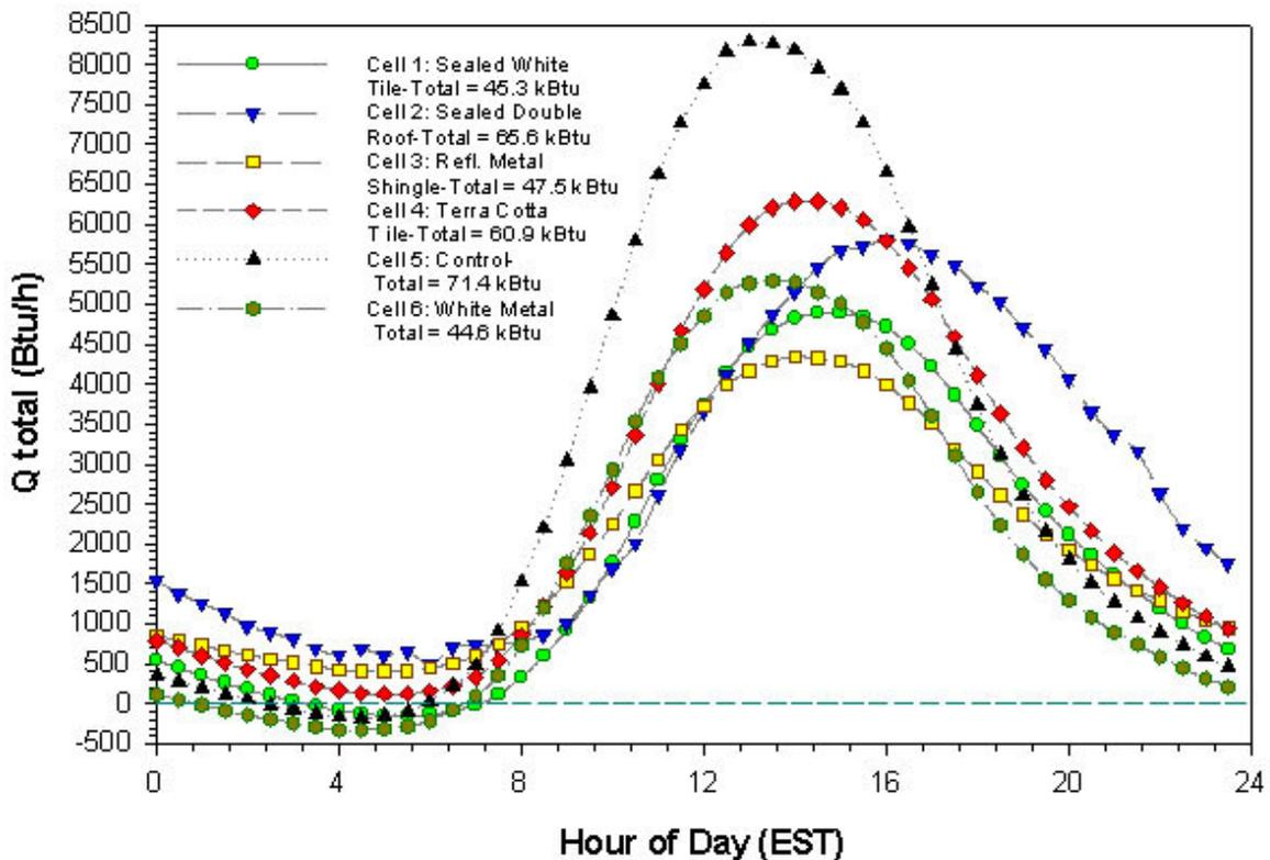
**Figure 8.** Estimated combined impact of duct heat gain, air leakage from the attic to conditioned space, and ceiling heat flux on space cooling needs on an average summer day in a 2,000ft<sup>2</sup> home.
