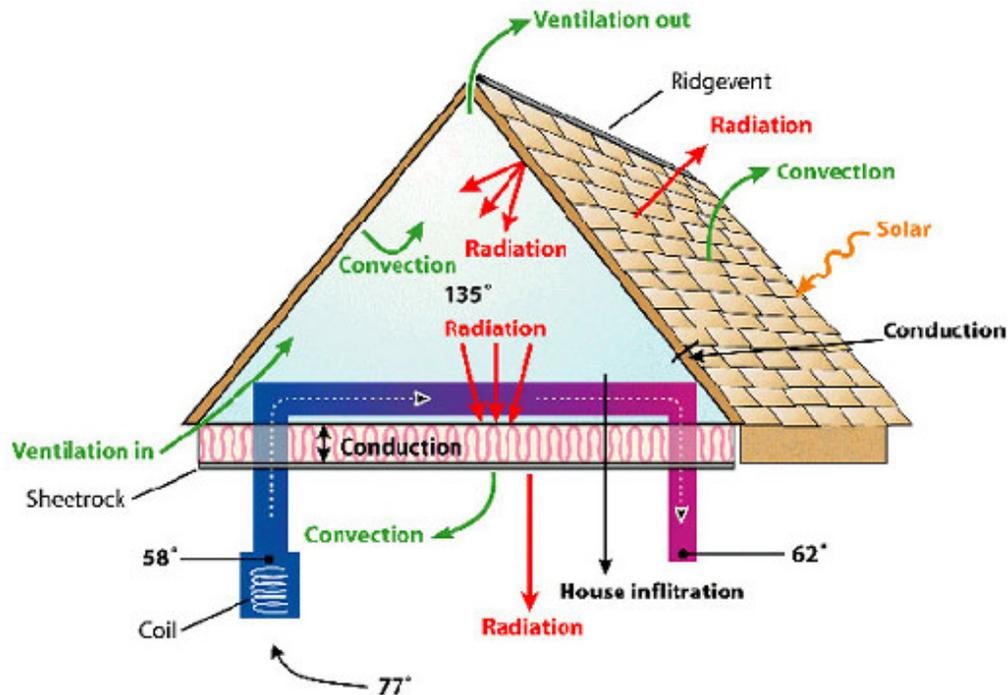
**Figure 1.** Vented attic thermal processes.
