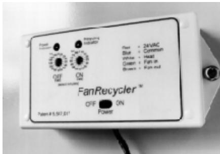
First commercially applied at the Prairie Crossing, Grayslake, Illinois development as part of the Building America Program, FanRecycler ([Figure 36](#)) is now a key component in central-fan-integrated ventilation systems in homes throughout the U.S. and Canada. More than 1,200 FanRecycler units are currently in use and it is available commercially from Shelter Supply, Inc. (Lakeville, MN).
