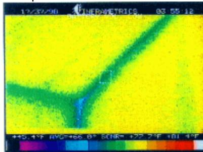
([Figure 35](#)). These infrared images indicate a small thermal short (the blue and green areas) which did not grow substantially after the house was depressurized.
