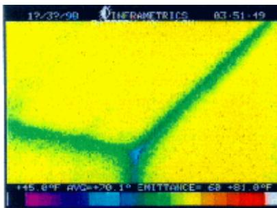
Infrared scans confirmed the low air leakage. While there were a few cold spots (e.g. near the floor behind the kitchen cabinets, at the intersection of windows and walls, wall corners, panel joints at gable ends etc.) as to be expected in any construction, the size of the cold spots did not increase when the house was depressurized. Infrared images show a very tight joint at the corner of the bedroom before depressurizing ([Figure 34](#)), and after five minutes at -50 pascals
