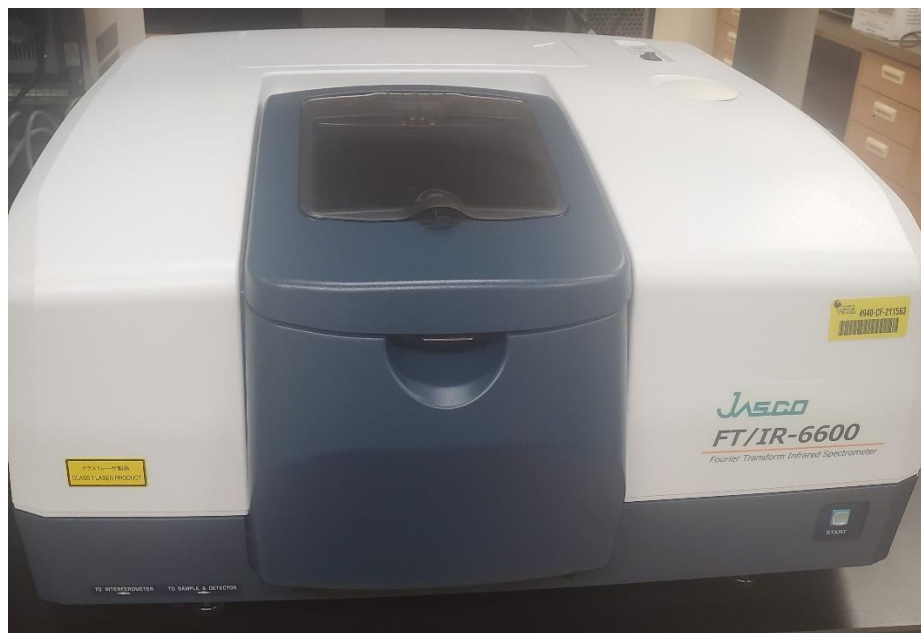
Figure 3.10: Jasco FT/IR 6600 spectrometer used to detect chemical bonding in the BCN thin films.
