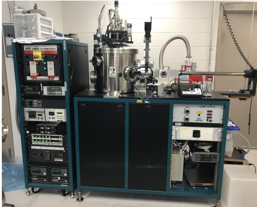
Figure 3.2: An AJA International 3-gun sputtering system used to sputter thin films of hydrogenated boron carbide.
