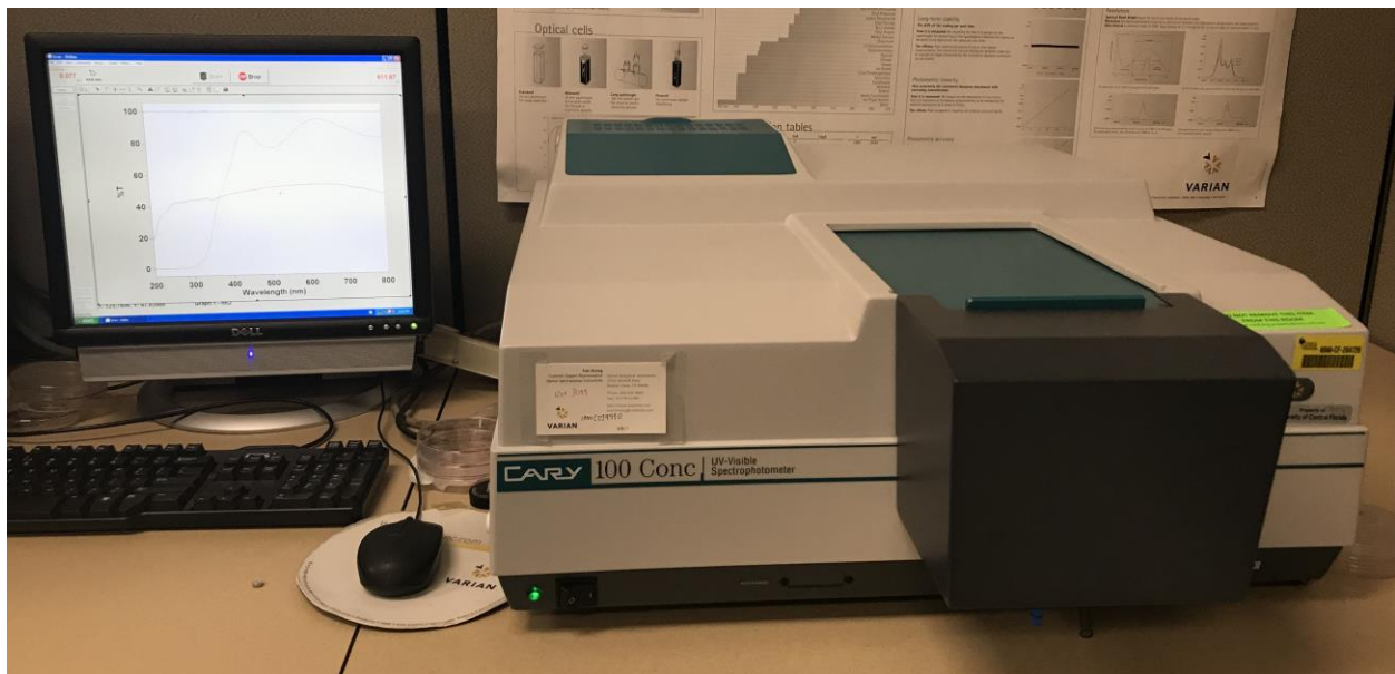
Figure 3.8: Cary 100 UV-Visible spectrophotometer used for optical characterization of thin films.
