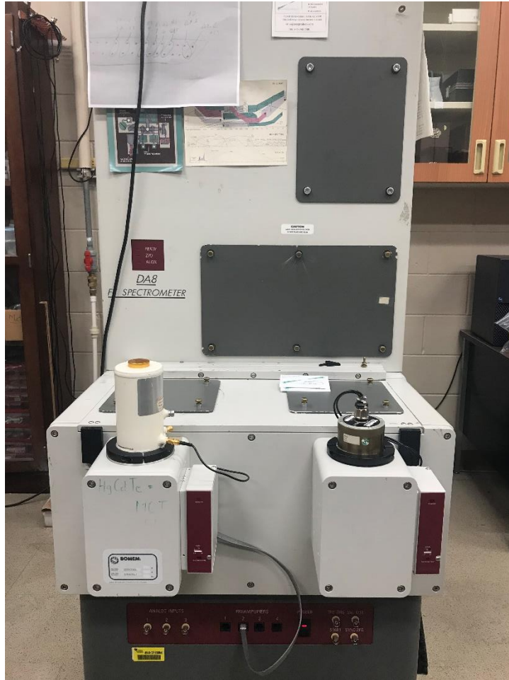
Figure 3.13: Vacuum bench BOMEM DA8 FTIR spectrometer equipped with MCT detector.
