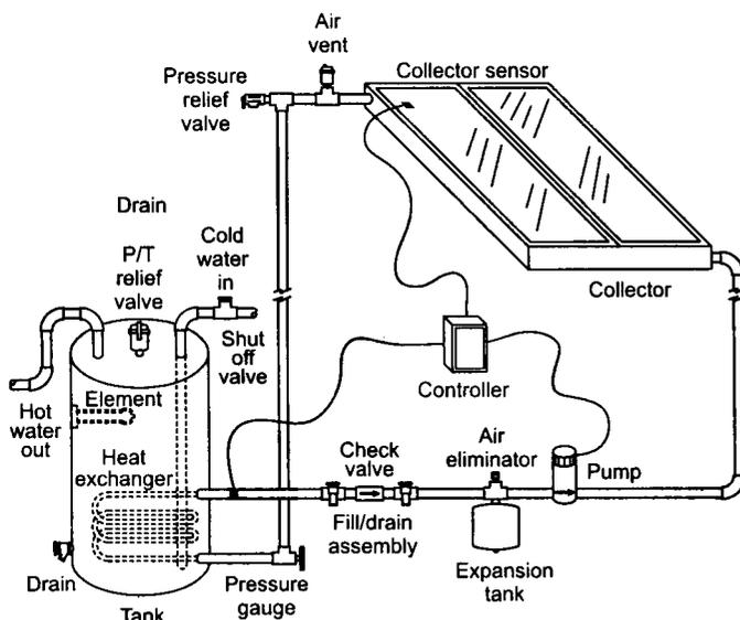
Figure 3. Indirect pumped system using antifreeze solution
