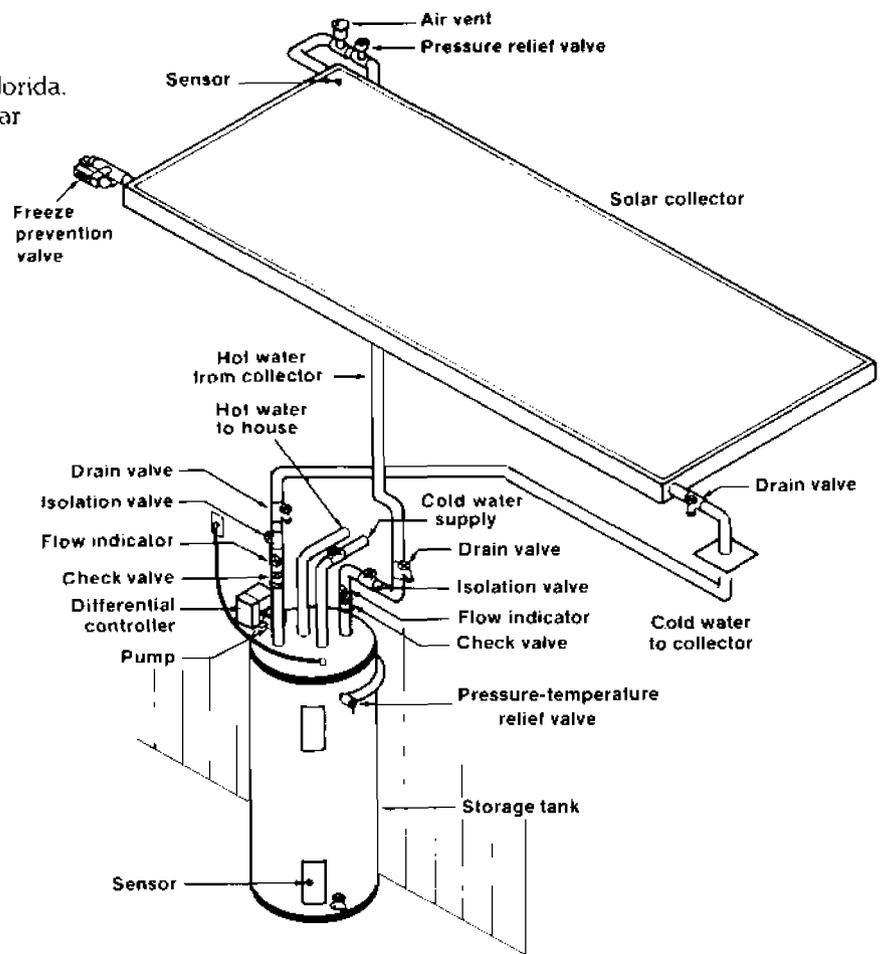
Figure 1. Typical direct pumped system.
