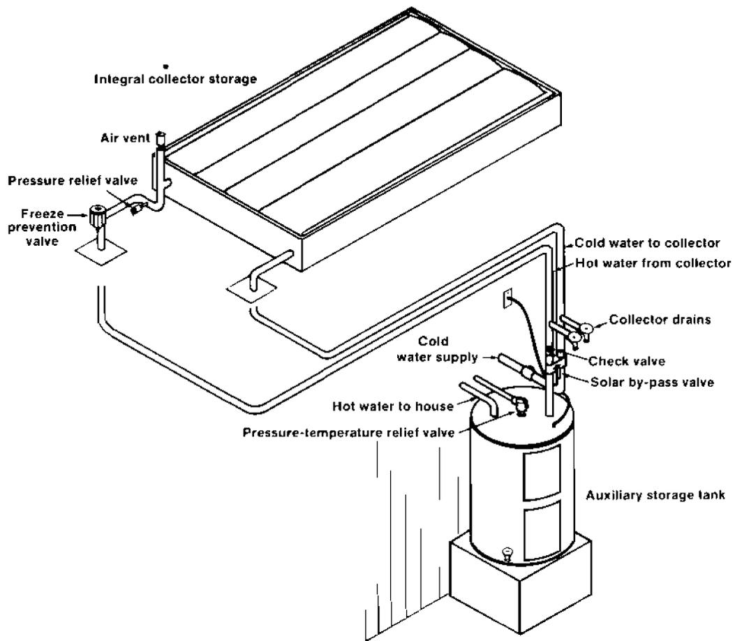
Figure 6. Integral collector storage system.
