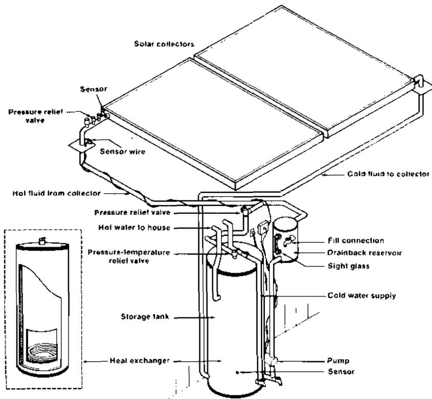
Figure 4. Indirect system using distilled water.
