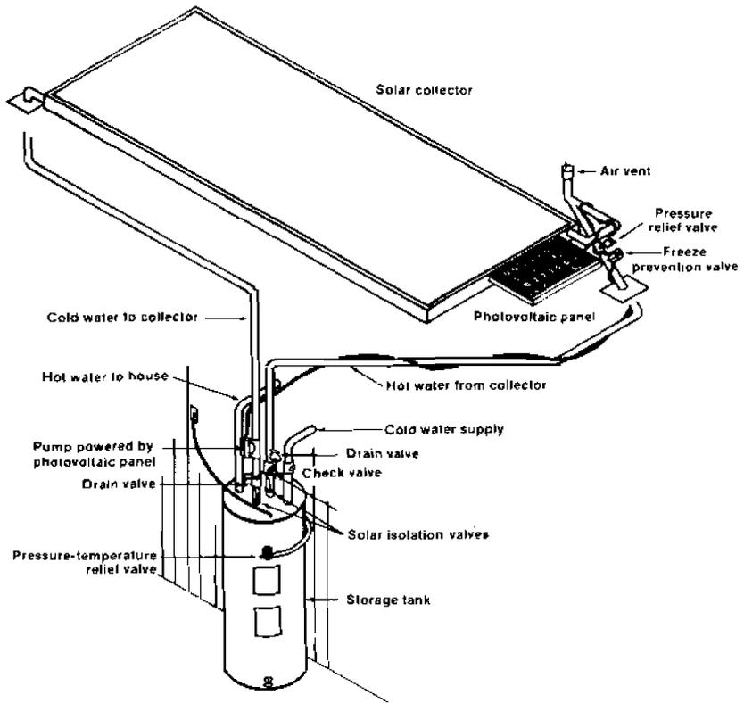
Figure 2. Direct system with photovoltaic-powered pump.
