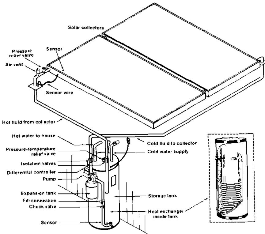
Figure 3. Indirect pumped system using antifreeze solution.
