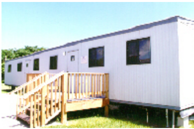
Figure 1. The Daylighting Test Facility (DTF) was used to collect data on offices with windows, blinds, and daylight dimming ballasts.
