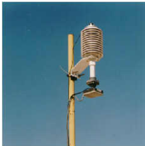
Figure 7. Ambient and relative humidity air temperature measurement configuration; silicon cell pyranometer is mounted on top.
