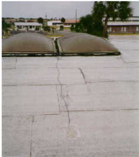
Figure 8. Roof surface temperature thermocouple on modified bitumen surface. Other thermocouples below measure decking and roof plenum space temperatures.
