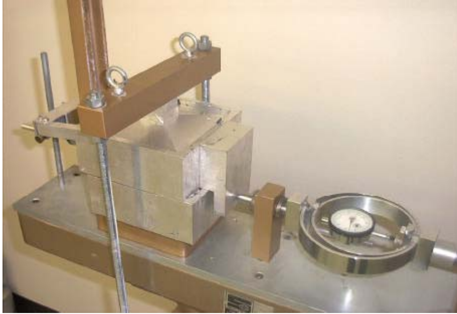
Figure 10: Shear box assembly for Direct Shear test
