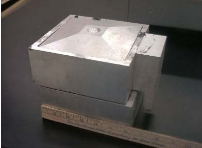
Figure 9: Large size direct shear test box
