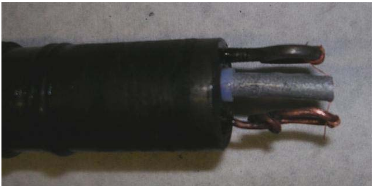
Figure 5: Propellant Strand Prepared in Strand Holder
