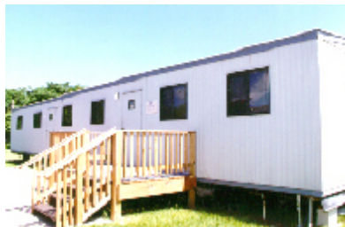
Figure 2. The Daylighting Test Facility (DTF) was used to collect data on offices with windows, blinds, and daylight dimming ballasts.
