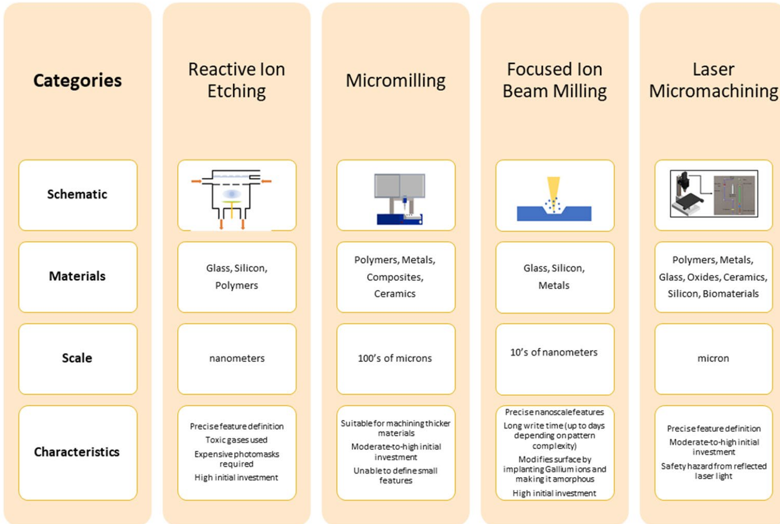
Figure 1 Comparison of three widely used direct-write fabrication methods (RIE [49, 51], micromilling [48], and FIB [47,50,53]) to laser micromachining. Each of these methods allows for high aspect ratio, serial, single-substrate fabrication. In the case of RIE multi-wafer/multi-substrate parallel processing is also possible as with some laser micromachining examples as well for higher throughput micro/nanofabrication.
