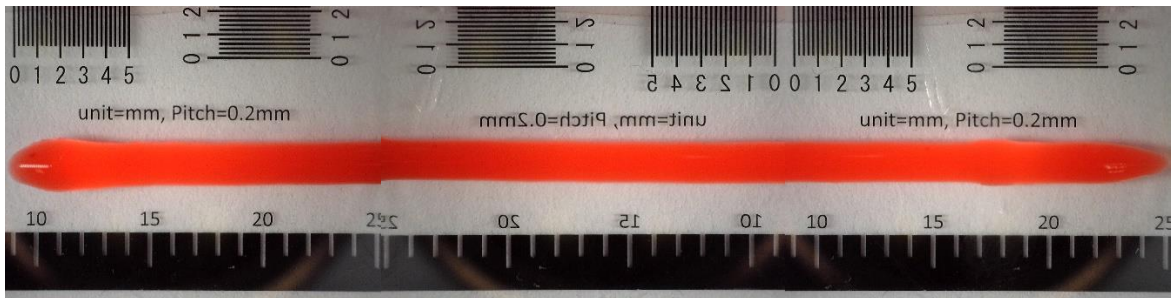
Figure 20: Dino captured image of extruded bioink at high pressure and low speed
