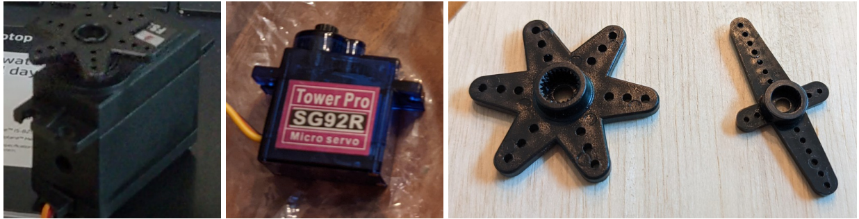
Figure 5.23: Here we show the Longrunner LKY62 continuous servo and the TowerPro SG92R standard servo experimented with, both of which came from Adafruit Industries (2005) . The TowerPro servos were ultimately used for this work. The rightmost image shows available horns that were used to connect the servos to the triangular unit facade discs.
