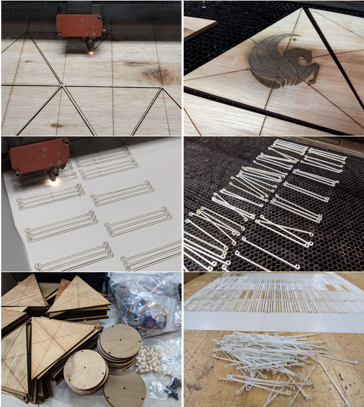
Figure 5.21: Here we show various photos of the laser-cutter at work on sheets of lauan plywood and acrylic. All triangular unit centers, backs, “wings,” discs, and connecting rods were cut with a Universal Laser Systems ILS12.150D laser-cutter. Our Rhino designs provided holes in the discs and centering markings per wing to save us time during assembly.
