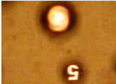
Fig. 5. Two different liquid lenses driven from focus (defocused) state to defocused (focus) states. ( Media 1 ).
