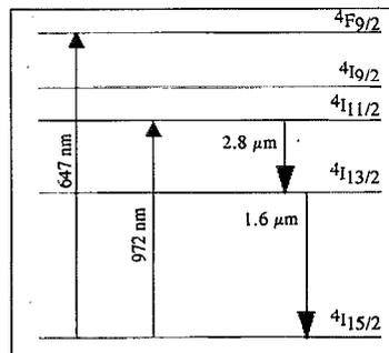
FIG. 1. Erbium-energy-level diagram.
