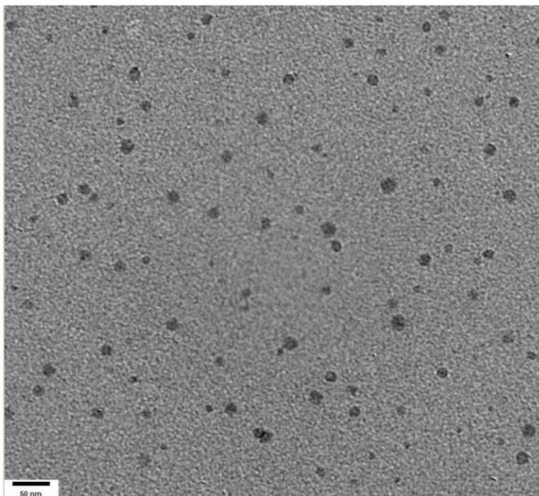
**Figure 10.** Transmission electron microscopy image of a PAA-Dopamine nanoparticles at 317.2kx magnification.
