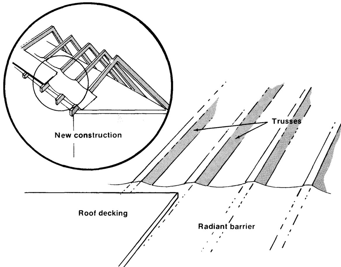
**Figure 5. Radiant barrier installation in new construction.**
