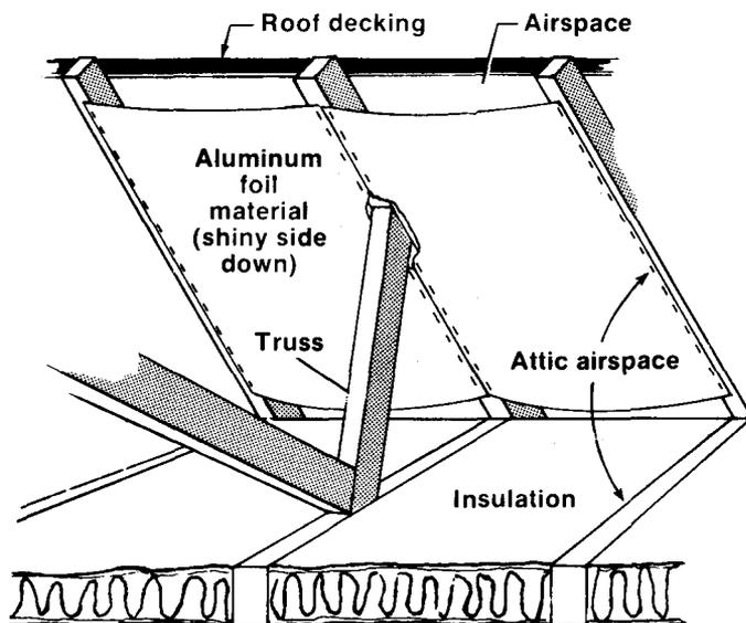
Figure 1. An installed radiant barrier.
