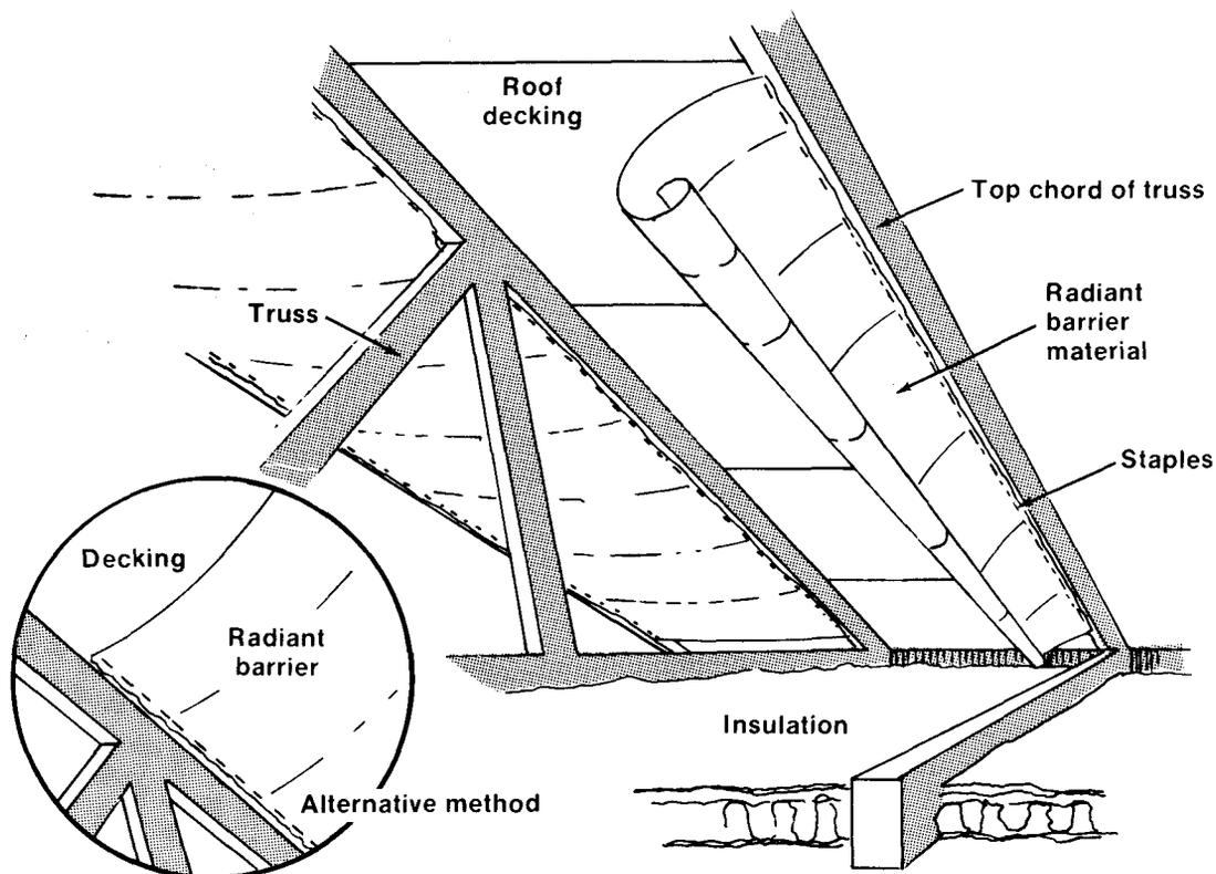
Figure 3. Locations for radiant barrier materials.
