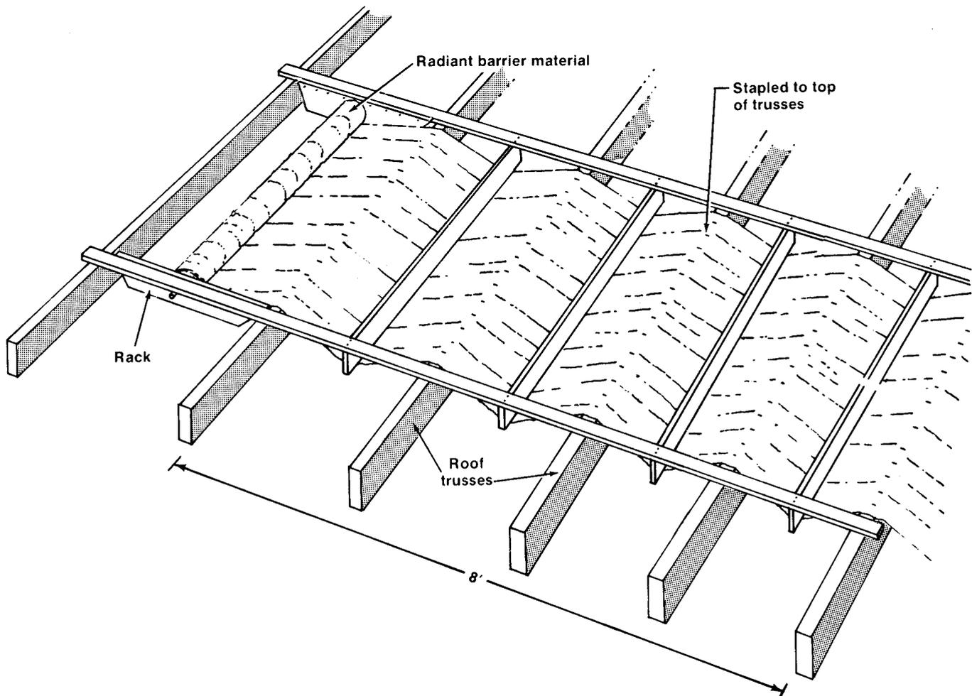
Figure 6. Installation rack.
