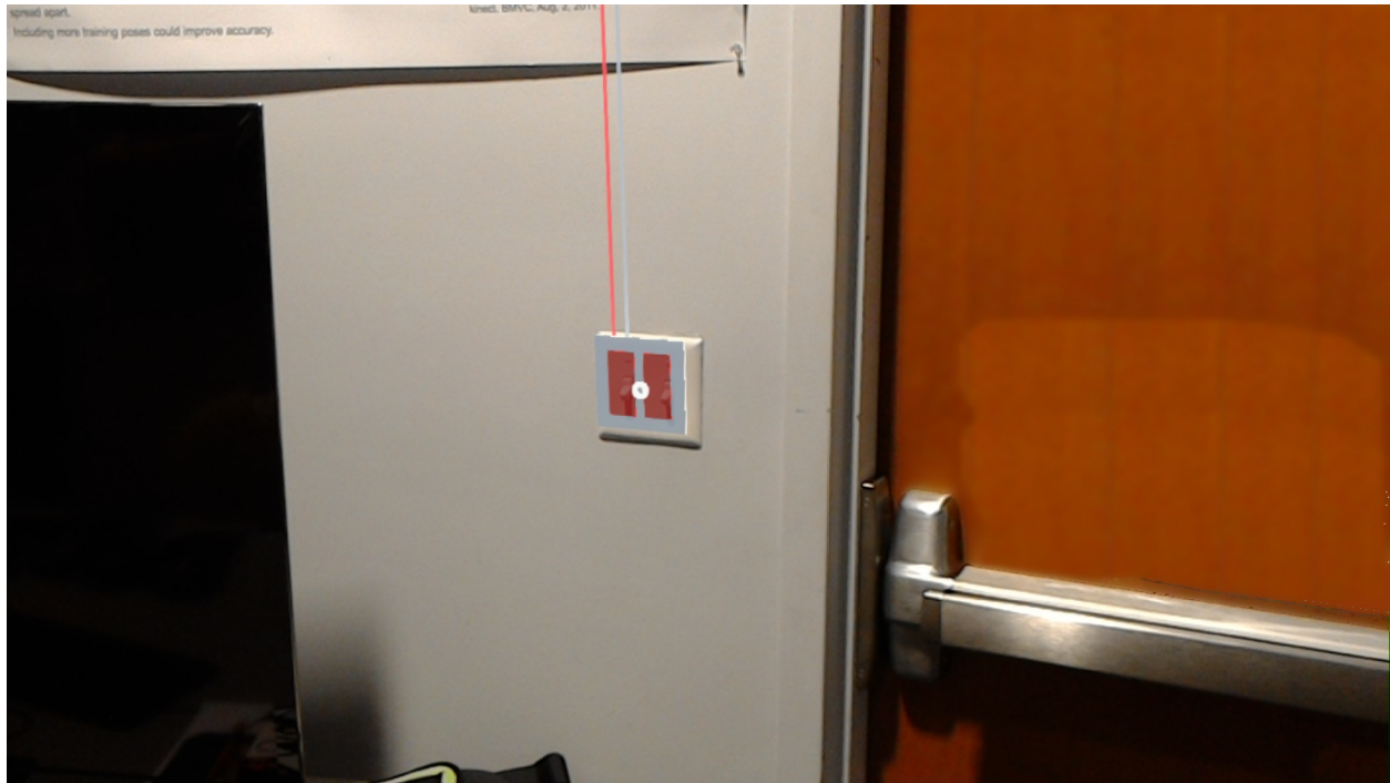
Figure 3.4: AR capture of the headset presenting a light switch which overlays a real switch and shows the parallel circuits running to the ceiling lights.
