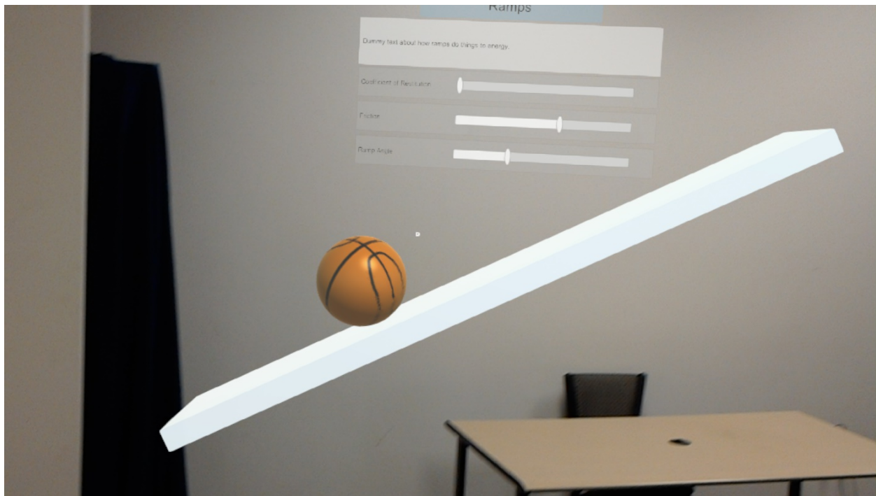
Figure 3.3: Capture of the AR headset presenting a ramp with a bouncing ball, which interacts with the spatial mesh captured by the HoloLens.
