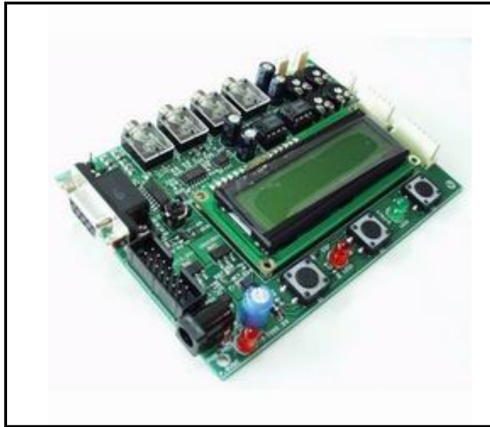
Figure 13 Olimex Development Board
