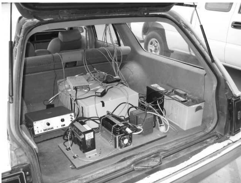
Figure 43 – Rear shot of Station Wagon Cargo Area Showing Mobile PC and Other Equipment.
