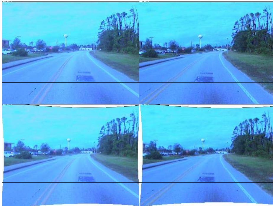
Figure 58 – Example of Rectification of Stereo Pair
