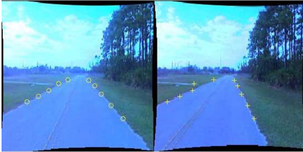
Figure 67 – Matching Points Between Left and Right Road Images
