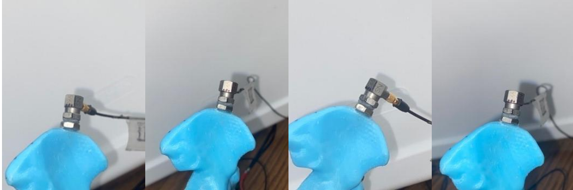
Figure 40. Demonstrated loosened sensor III coupling by 15 degrees within a single set (0 > 15 > 0 > 15)
