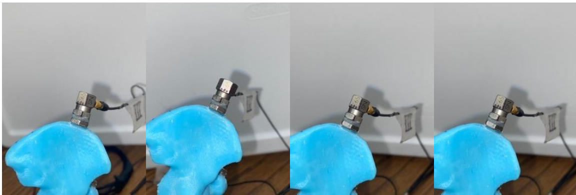
Figure 41. Demonstrated loosened sensor III coupling by 30 degrees within a single set (0 > 30 > 0 > 30)
