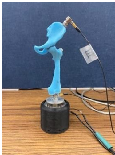
Figure 22. General experimental setup for loosened sensor II coupling.
