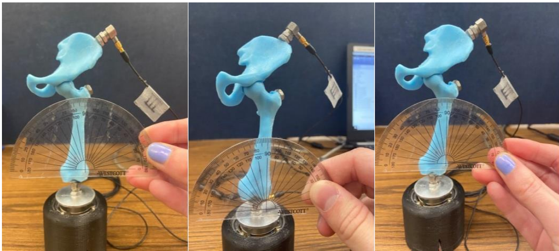
Figure 56. (left to right) Experimental setups for altered vertical femur alignment at 0 degrees, 2.5 degrees, and 5 degrees to the lateral.
