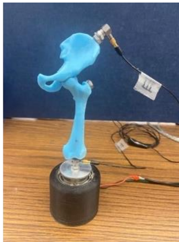
Figure 39. All of the experimental setups demonstrated looked like the picture shown. The only alteration was the rotation of sensor III on the top to loosen coupling of the accelerometer.
