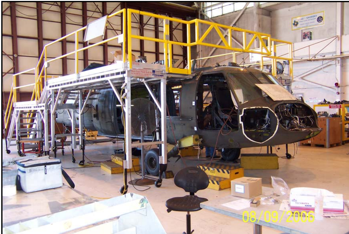
Figure 4: UH-60A Undergoing Structural Upgrades
