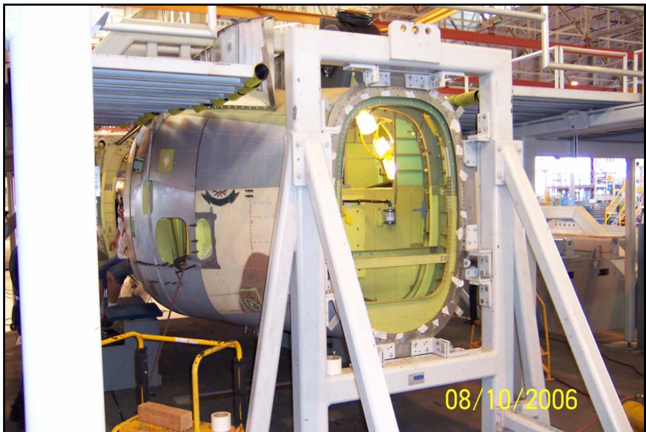
Figure 3: UH-60A Aft View with Tail Boom Detached
