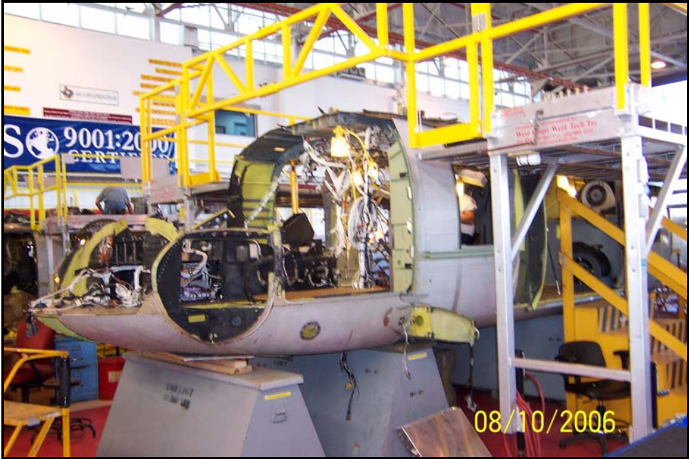
Figure 2: Forward View of Electrical Upgrades to UH-60A
