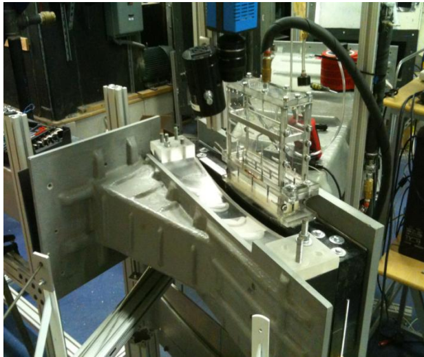
Figure 27: Film cooling section installed in cascade [1].
