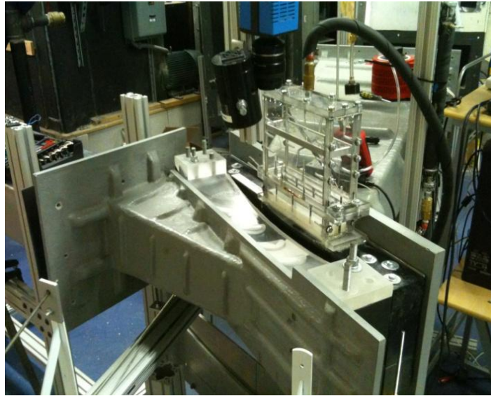
Figure 48: TSP setup on E 3 cascade [1].
